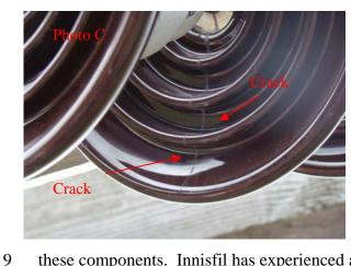
40 dead-end porcelain insulators are scheduled for replacement in 2009 within a multi-year replacement plan. These porcelain insulators are approximately 30 to 40 years old. At that advanced age, the dead-end porcelain insulators are cracking and tracking to the steel cross-arms resulting in pole fires (See Photo C). Hydro One has issued an industry wide bulletin indicating the danger of
