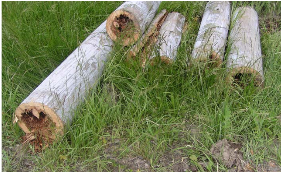
Figure 17, Pole decay in Grey Munsell Poles
