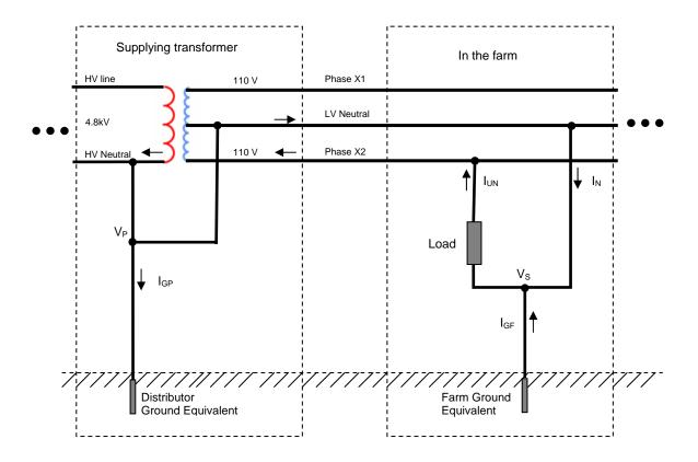
The above farm electrical circuits can be modeled as the following simpler circuits. A bad LV neutral connection is taken as the example here.
