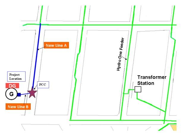
Example 3: Several Generators want to connect from Generator Sites on Private Property to a New Line that has to be built on Road Allowance to connect to the Main Dx System
