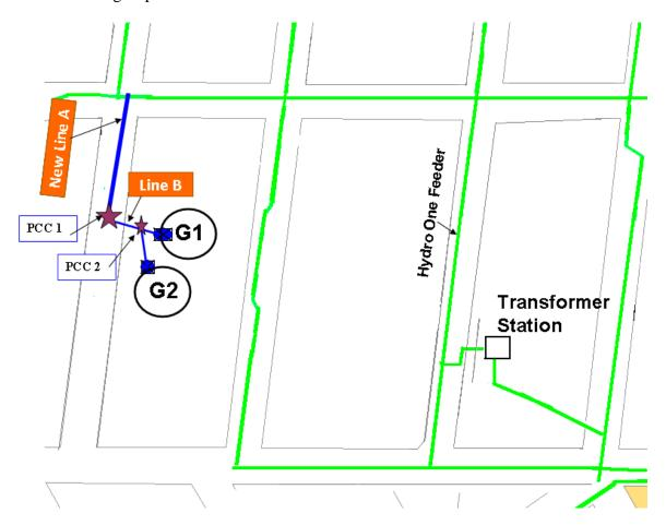
Example 5: One or More Generators want to connect from Generator Site(s) on Private Property to the Main Dx System and a Regulating Transformer needs to be replaced with a larger Regulating Transformer A to accommodate the connection
