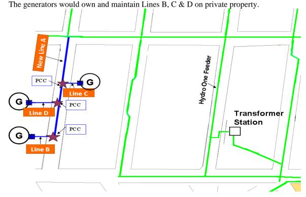
Example 4: One or More Generators want to connect from Generator Site(s) on Private Property to the Main Dx System and Existing Line A needs to be rebuilt to accommodate the connection
