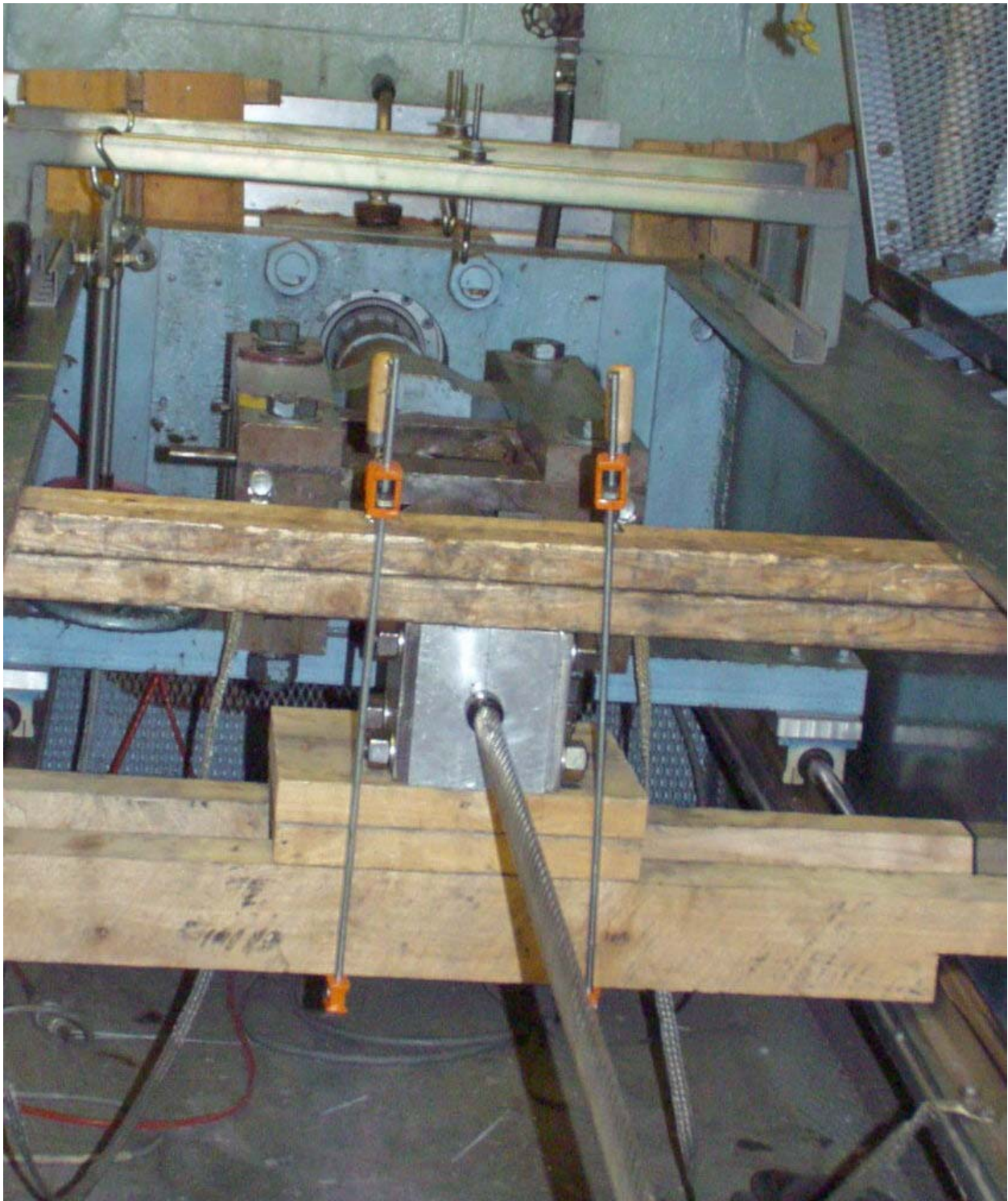
Photograph 3, cribbing used to prevent sample rotation
