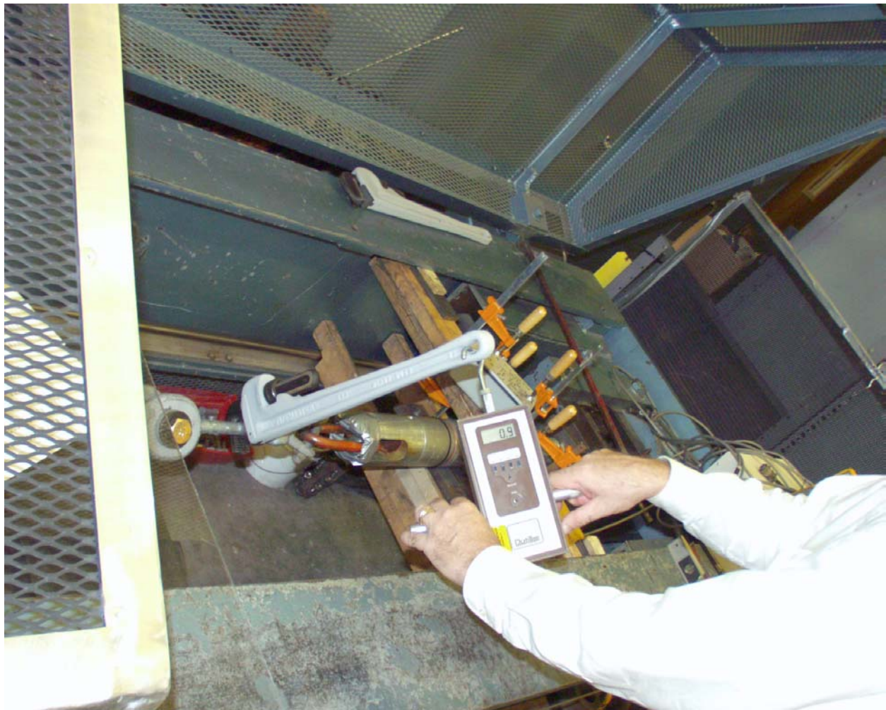
Photograph 1, sample rotation and torque measurement (note second pipe wrench)
