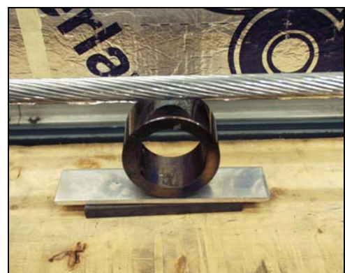
Photograph 3 Mid-span Support to Remove Sag
