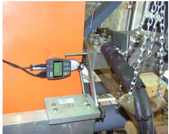
Photograph 2, Mitutoyo digital indicator, electrical connection, and rubber heat shield for gage rod
