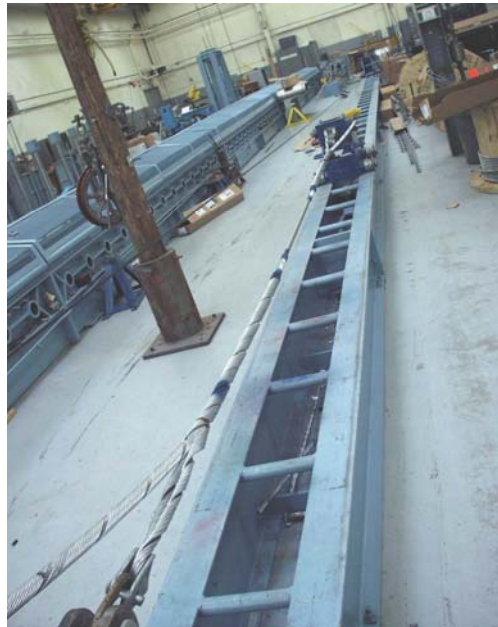
Figure 1. Test set-up for Tensile Test
