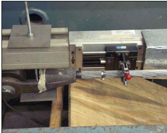
Photograph 2 Sliding Carriage and Linear Position Instrument (Conductor in photographs is not 596TW, but does illustrate the test configuration)
