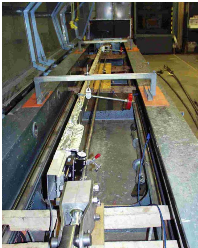
Long View of Stress-strain Test on 675/TW Conductor
