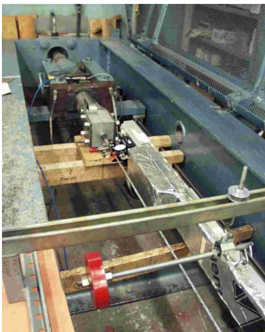
Photograph 2 Load Actuator and Extensometer (Core strand is under test)
