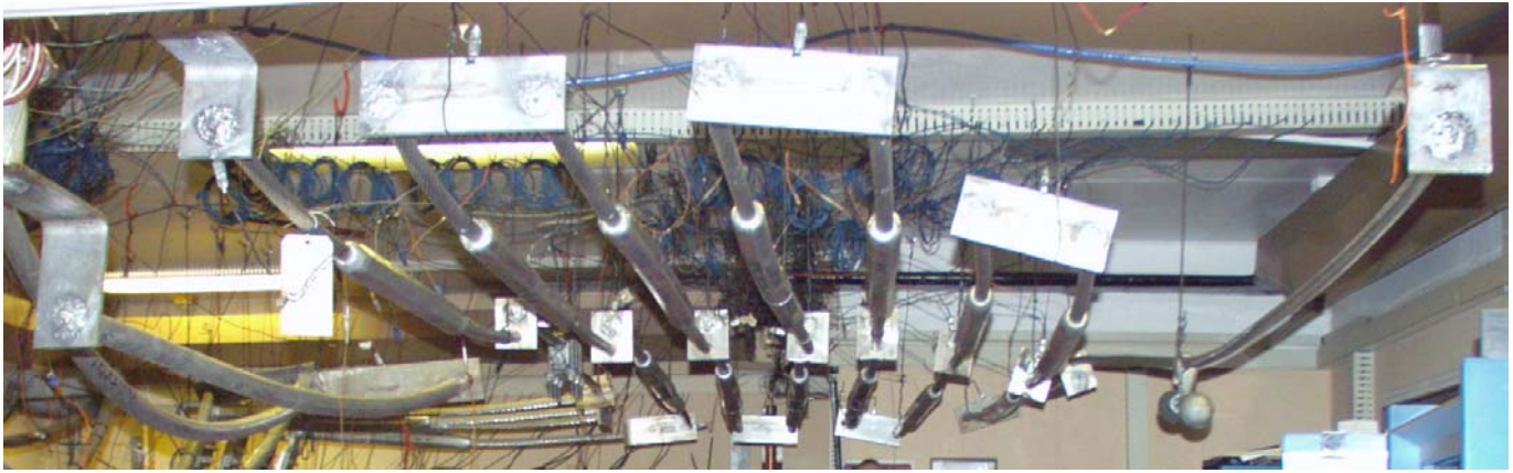
Photograph 1 795 kcmil 3M Composite Conductor connector test loop
