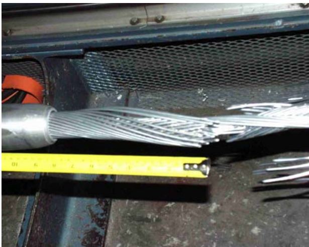
Photograph 3, Gage section break
