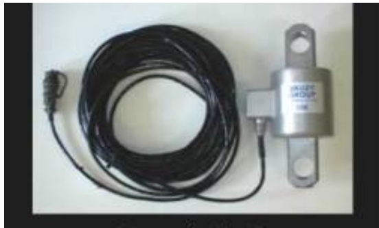
A- Load cell used to measure tension
