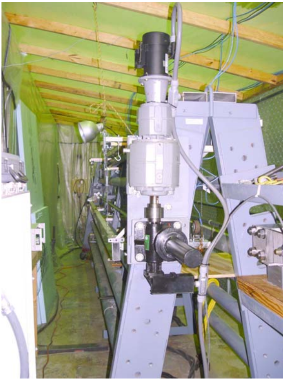
Photograph 1, long view of creep frame showing lead screw drive
