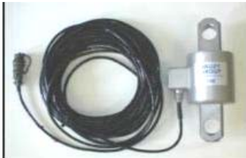
5-a Load cell to monitor tension
