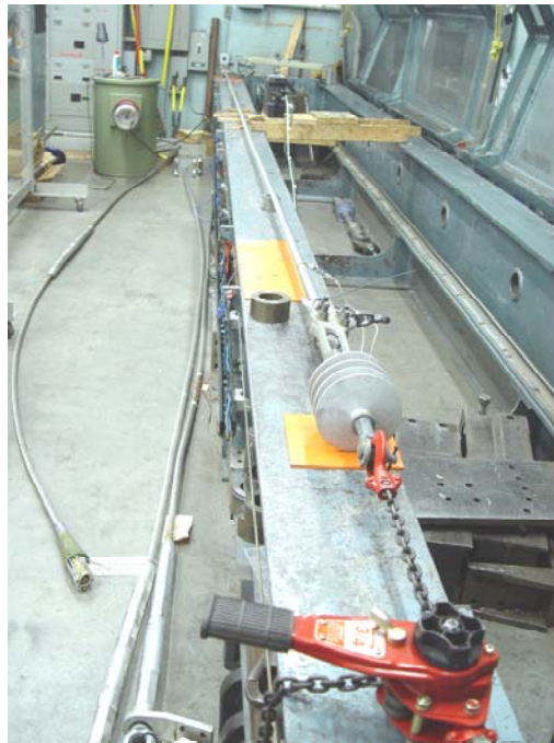
Figure 27- Resistance measuring set up and sample
