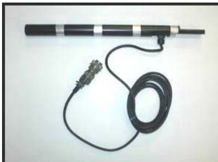
5-c Net radiation sensor, Measures no - load conductor temperature and solar radiation
