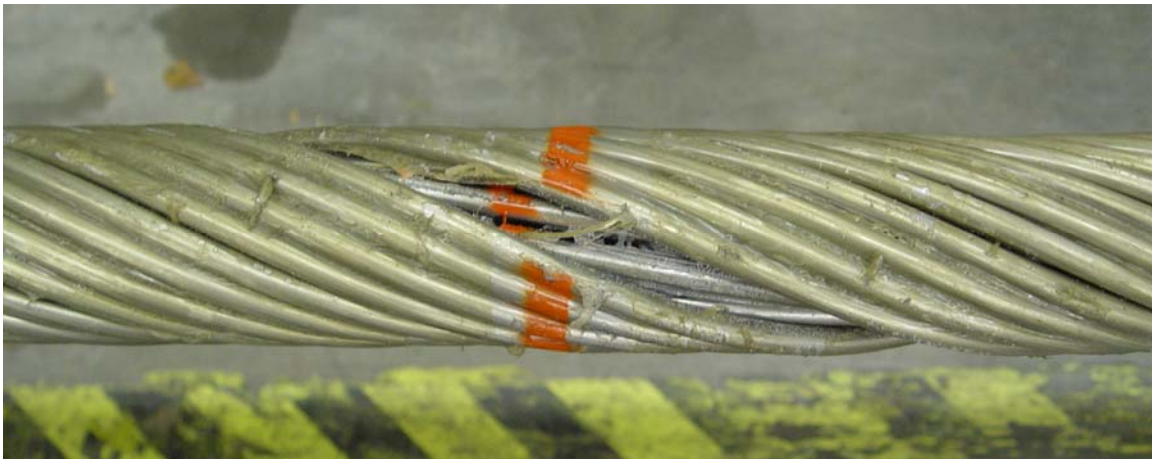
Figure 34: outer rods shifted under load
