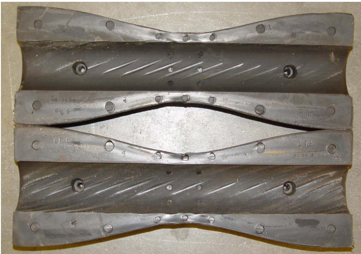
Figure 29: Inside of rubber conductor cushion is also in good condition
