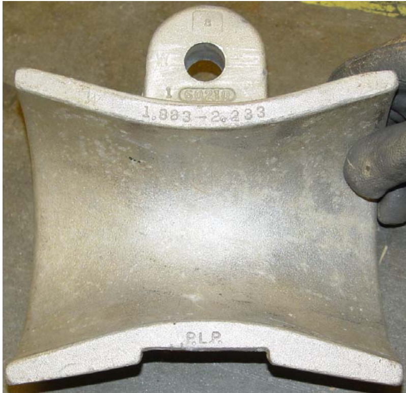
Figure 30, Metal housing is in good condition after field test
