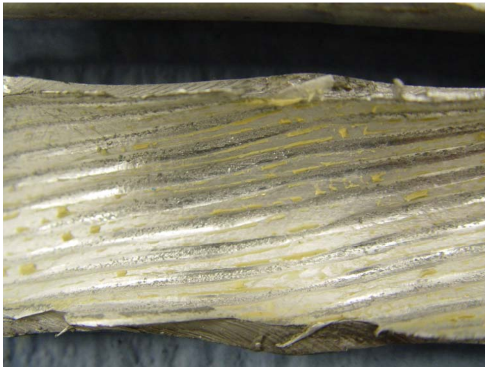
Figure 21: Conductor OD shows no evidence of wire-brush marks
