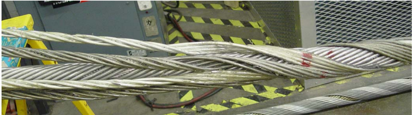
Figure 38: rods shifted during service and tensile test, but break occurred elsewhere
