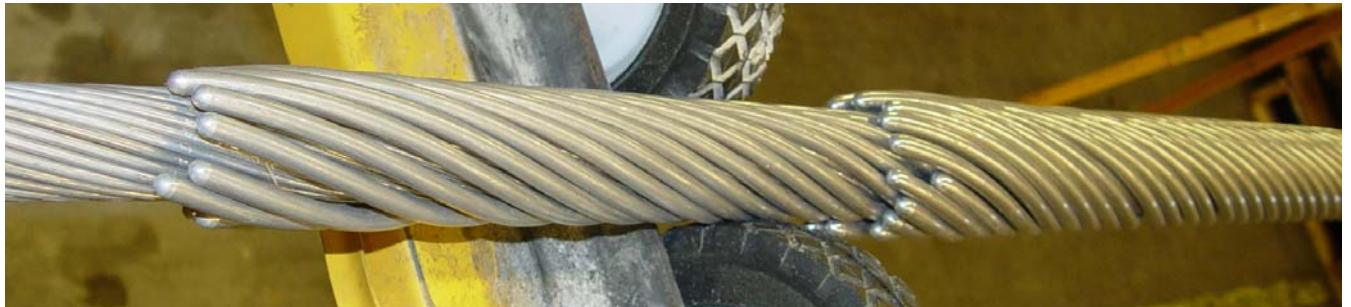
Figure 31, Formed wire rods slipped somewhat out of alignment, but the system appears to tolerate less than perfect installation
