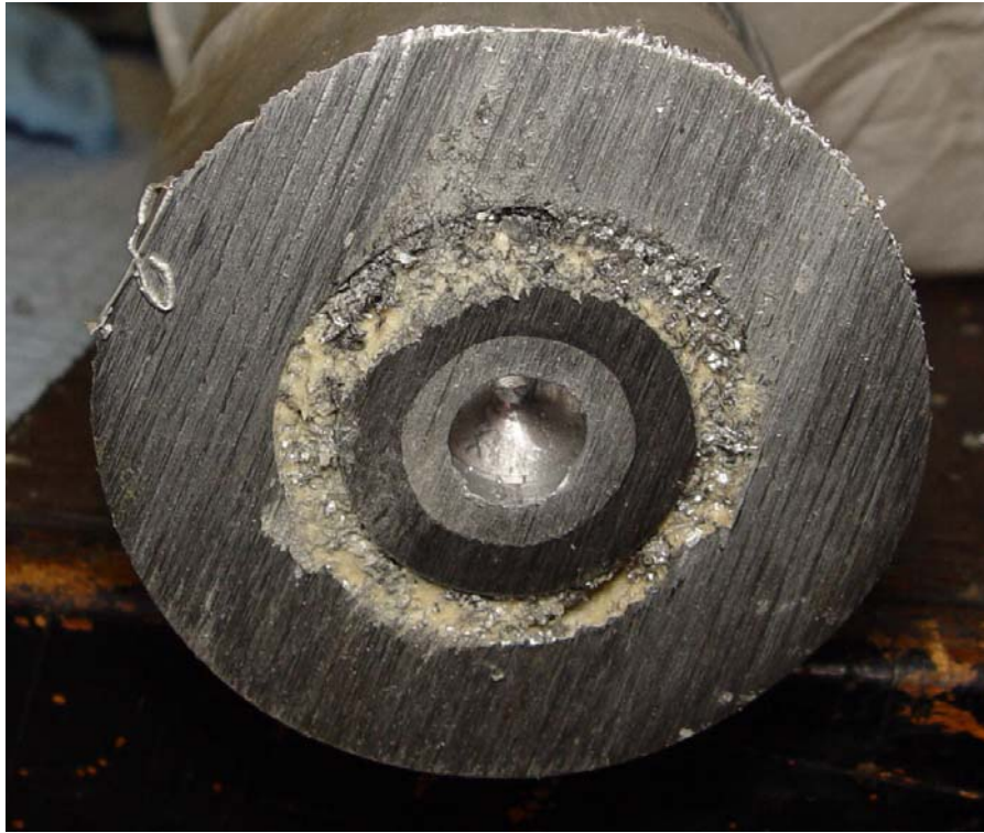
Figure 25: End of core sleeve. The core was inserted up to approximately 3/8 inch from the end of the bore.
