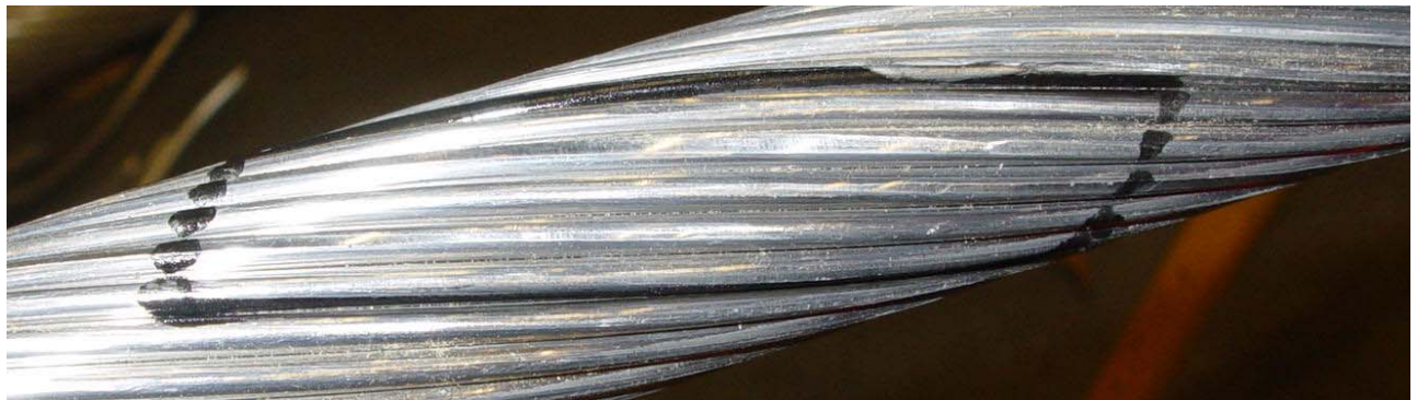
Figure 32, inner rods sustain imprint from outer rods, but underlying conductor is not harmed
