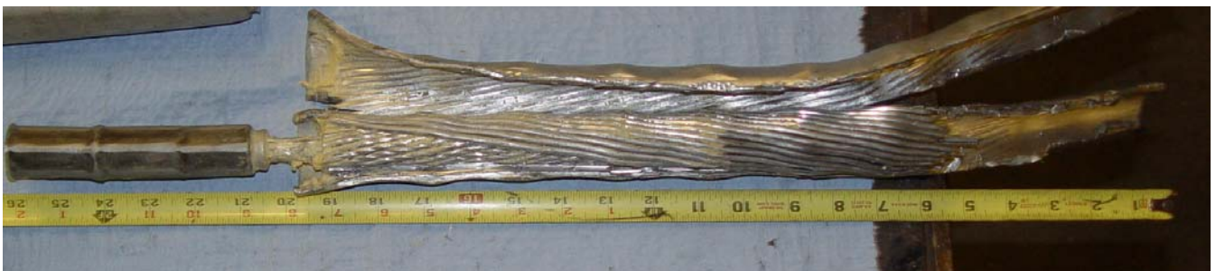
Figure 24: Inhibitor stops approximately 10 inches from mouth of dead end. Proper inhibitor charge should fill all conductor interstices to block water migration into the splice internals.
