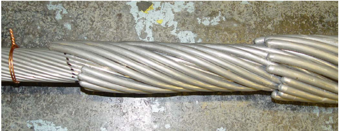
Figure 5, photograph of PLP splice after tensile test. Note rod slippage.
