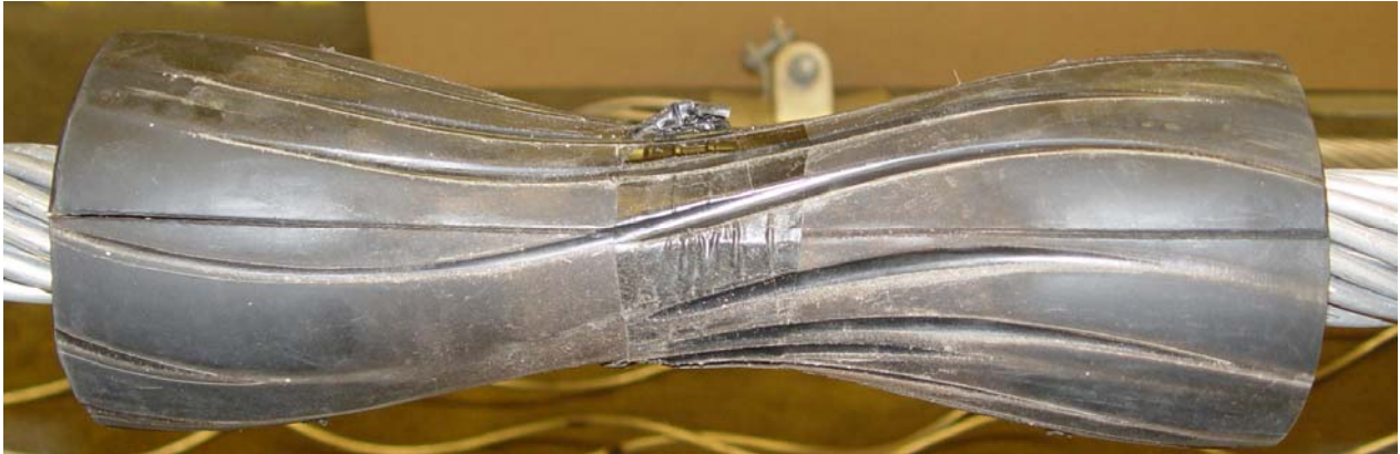
Figure 28: OD of rubber conductor cushion is in good condition
