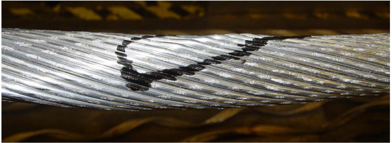
Figure 40: slight birdcaging of conductor strands under inner rods of PLP dead end after reaching 108% RBS in the tensile test
