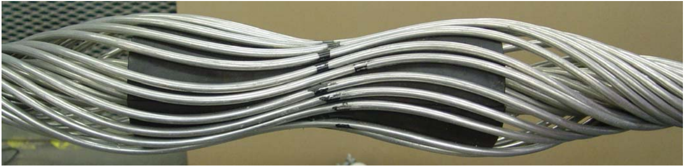
Figure 27: center marks on rods are not aligned, but there is no evidence this caused any problems
