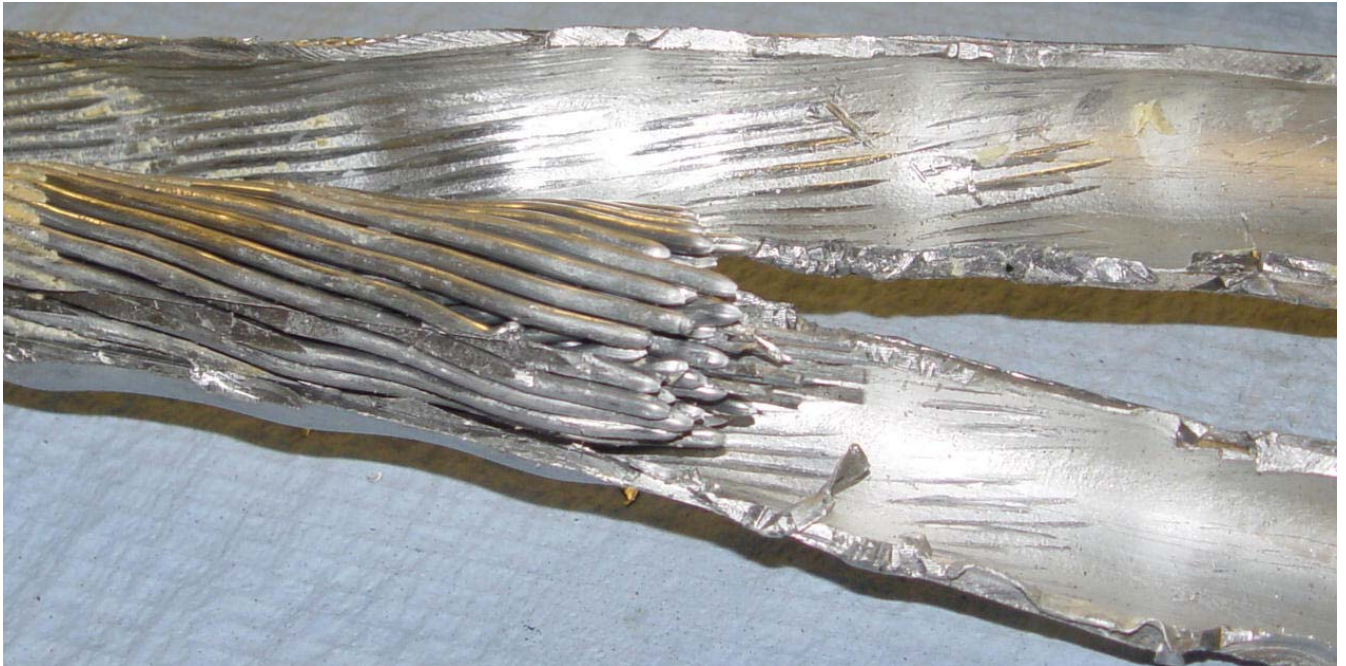
Figure 23: lack of inhibitor charge filling conductor shows fill port was not completely filled. Also note conductor has no evidence of wire brushing.
