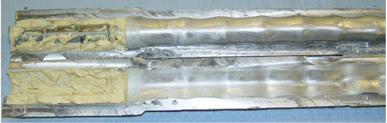
Figure 22: inhibitor charge at core sleeve shows injection port was used
