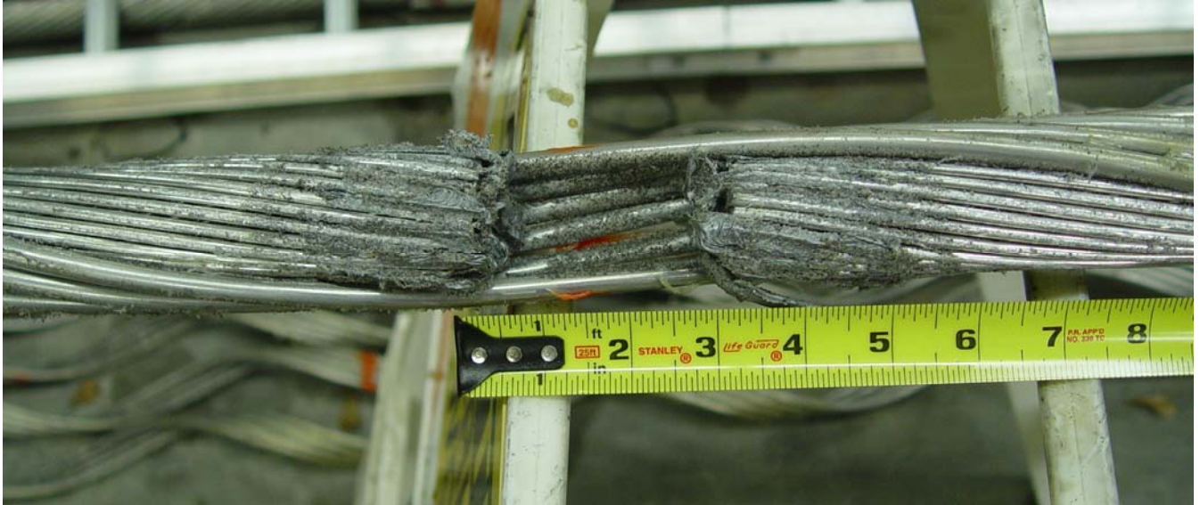
Figure 36: two inch gap between conductors inside the splice may be partly due to tensile test loads
