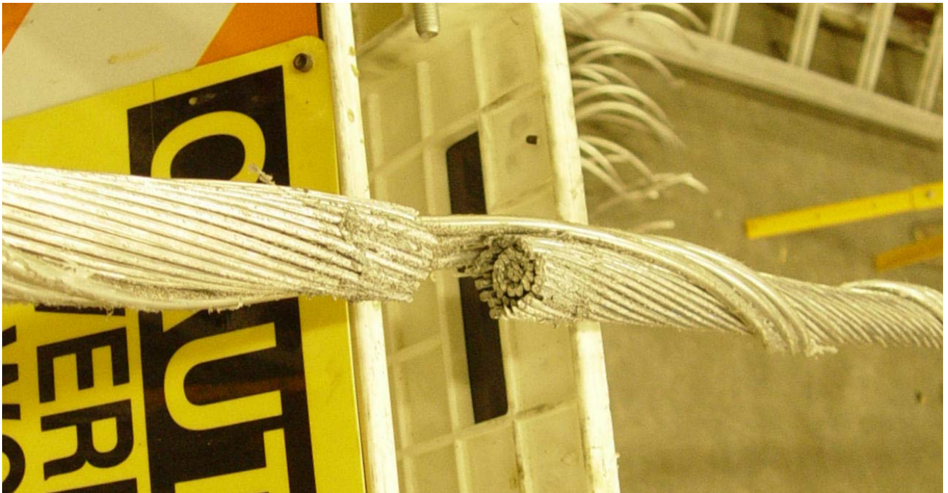
Figure 37: outer conductor strands are shifted due to tensile test load. Conductor broke in free-span section
