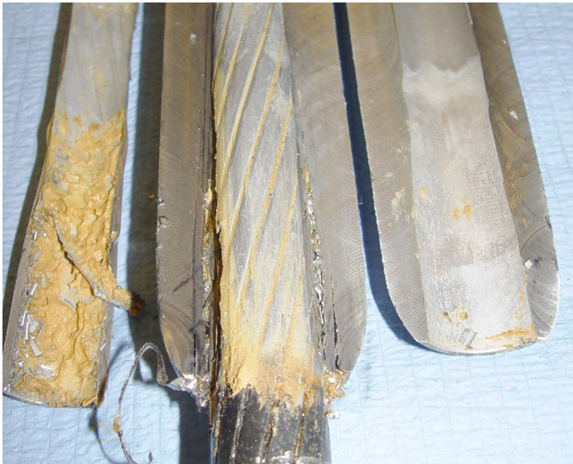
Photograph 5, exit from splice showing inhibitor on conductor OD
