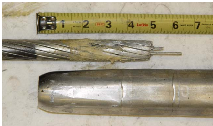
Photograph 1, splice sample after tensile test
