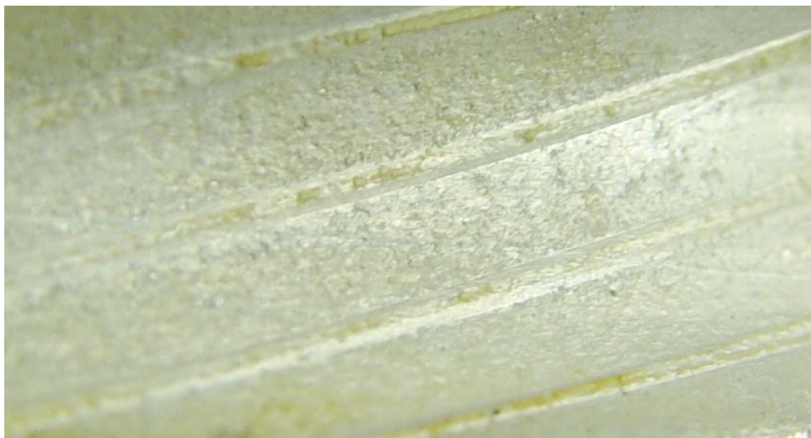
Photograph 7, close-up of conductor OD shows no evidence of wire-brush marks
