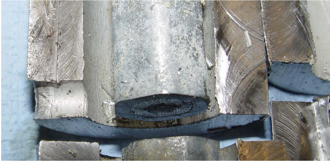
Photograph 4, splice cavity showing injection port. The plug was present, but there is no evidence that inhibitor compound was injected to fill the cavity
