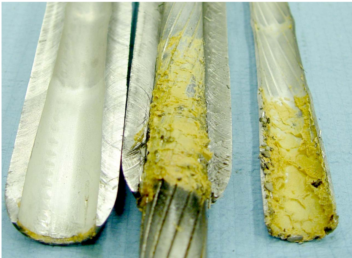
Photograph 6, opposite end of splice, again showing inhibitor only on conductor OD
