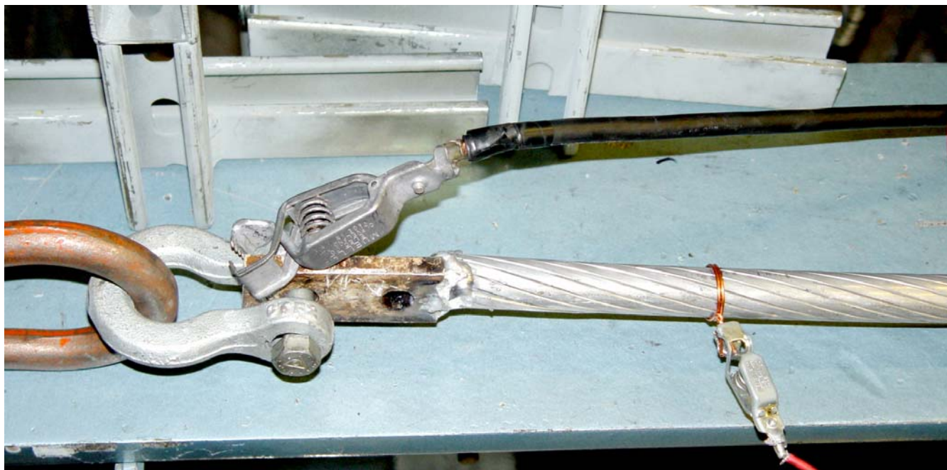
Photograph 2, current connection (left), and voltage connection (right), typical each end of sample
