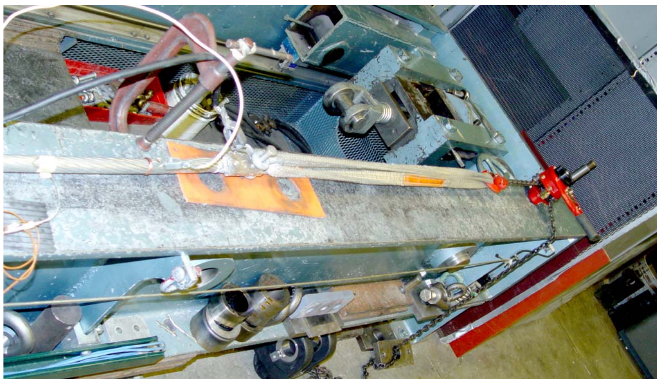
Photograph 3, resistance sample tensioning device, current, and voltage terminals (air gap, fabric strap and rubber pads ensure the sample is isolated)
