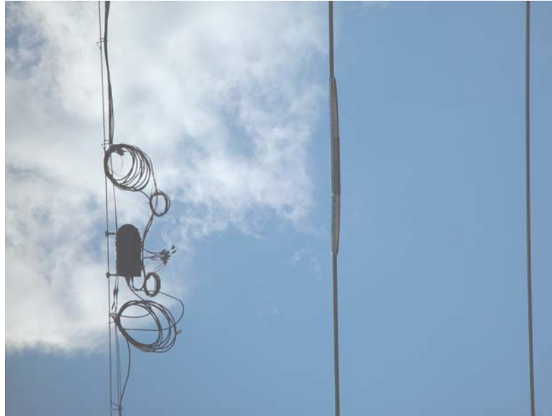
Figure 6 Thermocouples wiring for in-situ – temperature monitoring
