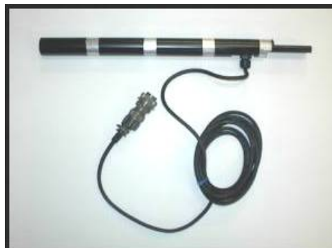
7- C Net Radiation Sensor Measures No Load Conductor Temperature
