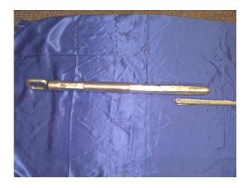
An example of an Alcoa Conductor Accessories compression dead-end which, failed at 19680 Lbs (101%RBS) inside the sleeve, near the tapered barrel.
