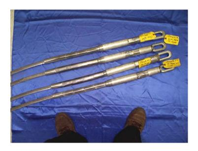
An example of a fully assembled, compression dead-end ready for testing, using the Alcoa Conductor Accessories two-piece dead-end approach.
