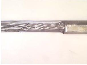
Section through a repair sleeve showing the cut Al strands at the center of the sleeve.
