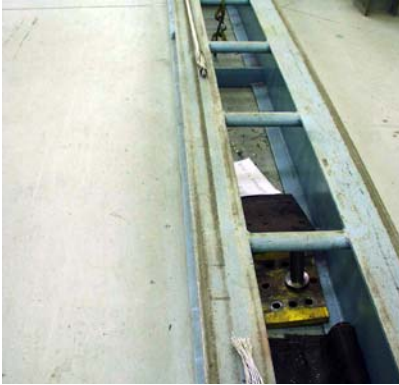
Figure 5 – Mid-Span Failure of Conductor
