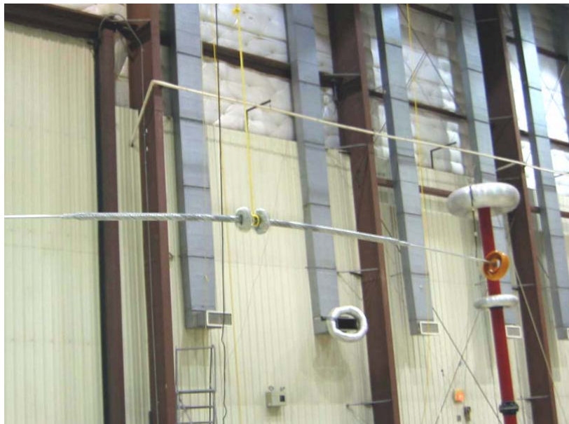
Figure 7 –Splice Arrangement in the Corona Test
