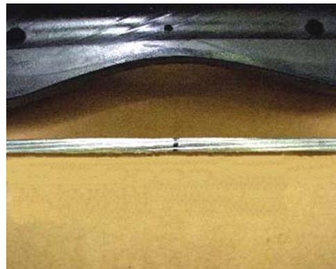
Figure 3 – Core After Aeolian Vibration Test
