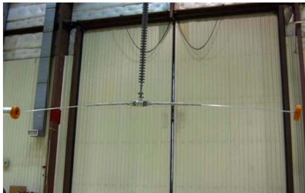
Figure 7 – Corona Test Arrangement for Suspension Assembly
