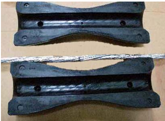
Figure 2 – Outer Strands & Aluminum Tape After Aeolian Vibration Test
