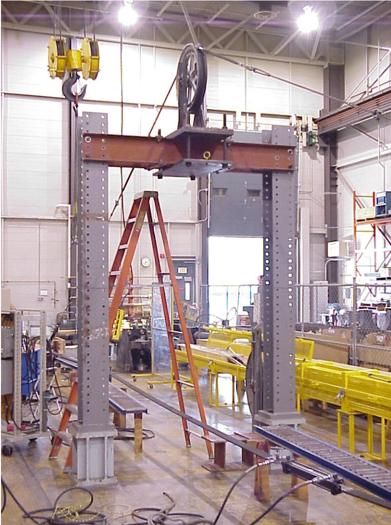
Figure 1d Typical Set-up for 16.75, 18, and 24 inch Single-Pass Sheave Test (24 inch Sheave shown in photo)
