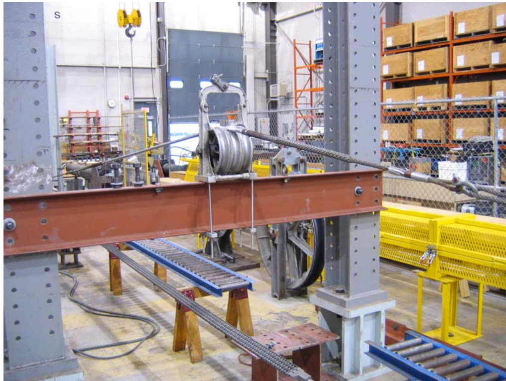
Figure 1b Typical Set-up for 8 inch Single-Pass Test
