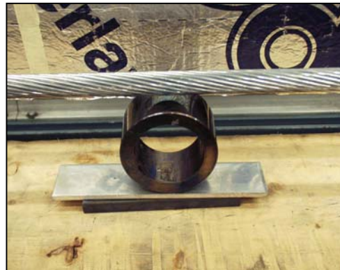
Photograph 5 Mid-span Support to Remove Sag
