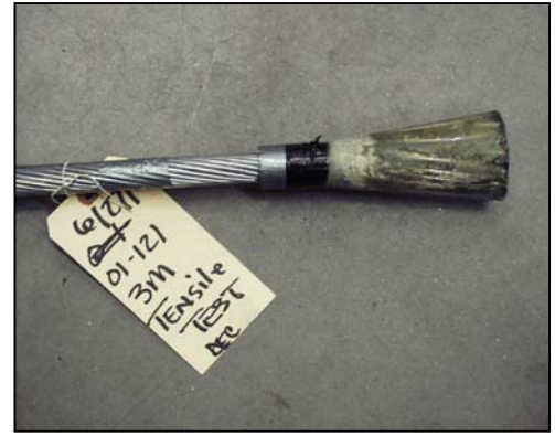
Photograph 2 Opposite Failed End (Resin Socket)
