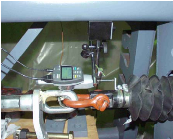
Photograph 1, Dead-end sample, load actuator, and dial indicator for actuator travel
