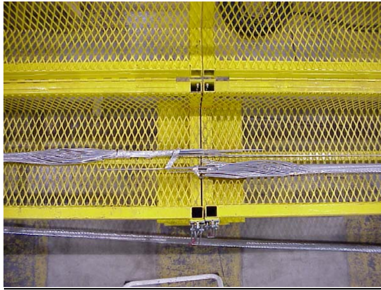
Figure 3 774-kcmil 3M™ Composite Conductor failure point after tensioning to failure. Conductor and Dead-end were stressed for 168 Hours while under Sustained Load at 240°C (Looking South)
