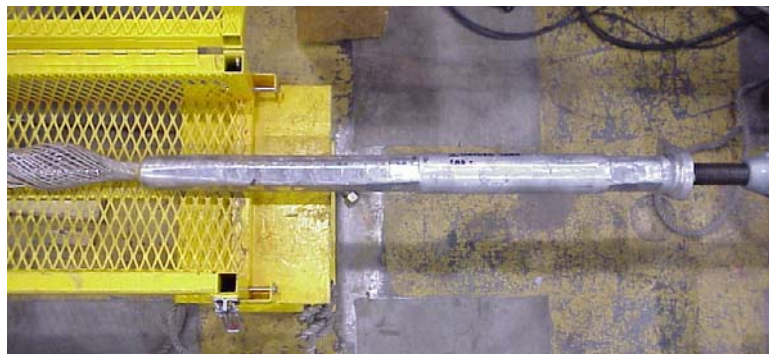
Figure 4 ACA Conductor Accessories Dead-end connected to a 774-kcmil 3M™ Composite Conductor after Tension to Failure. Conductor and Dead-end were stressed for 168 Hours while under Sustained Load at 240°C.
