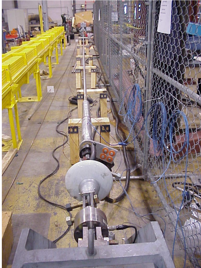
Figure 1 Set-up for Room Temperature Sustained Load Test of an ACA Conductor Accessories Dead-end connected to a 774-kcmil 3M™ Composite Conductor (Looking South)
