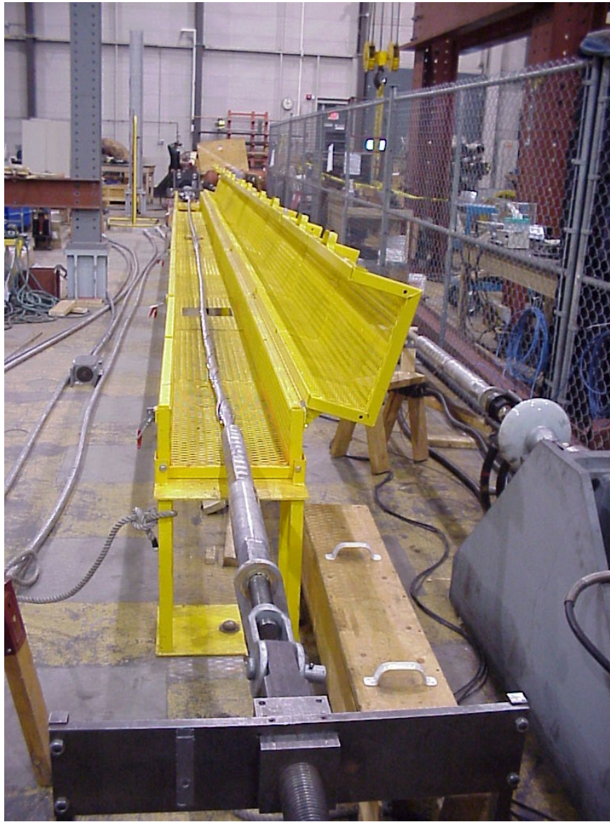
Figure 1 Room Temperature Sustained Load Test sample (post-test) of an ACA Conductor Accessories Deadend attached to a 774-kcmil 3M™ Composite Conductor (Looking South). Conductor and Dead-end were stressed for 168 hours under the Sustained Load at Room Temperature and then tested to failure in tension. Failure was at the mid-span.
