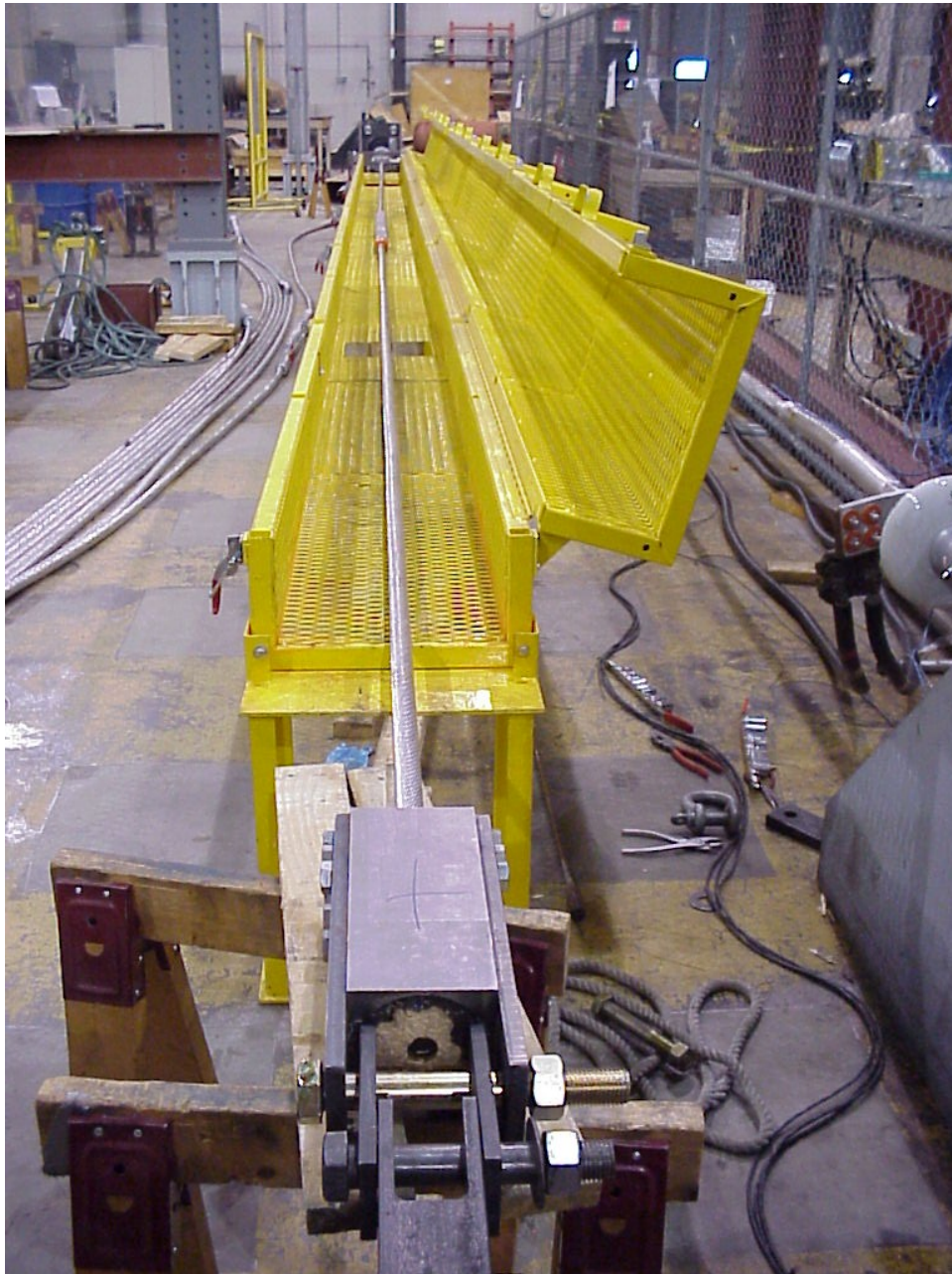
Figure 1 Set-up for Test on ACA Conductor Accessories 774-kcmil 3M™ Composite Conductor Full Tension Splice (Looking South)
