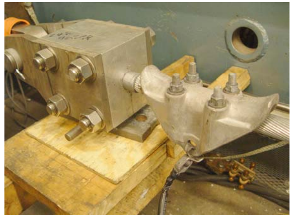
Photograph 2, bolted current terminal (2 places)
