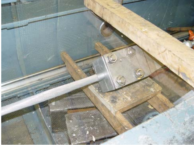
Photographs 6 and 7, initial bird cage after relaxing first negative torque cycle
