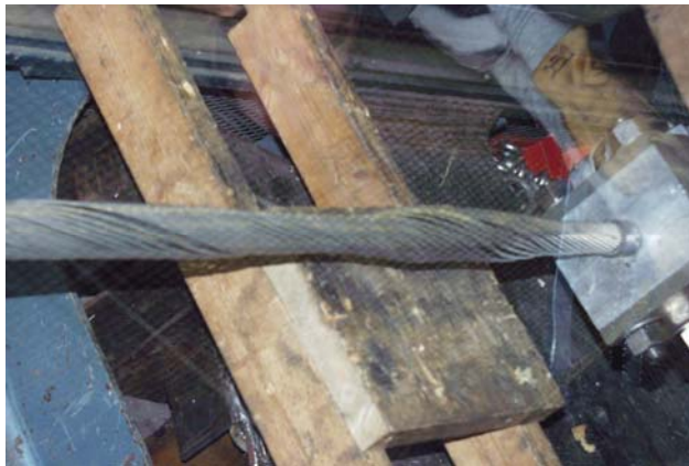
Photograph 10, conductor following torsion test
