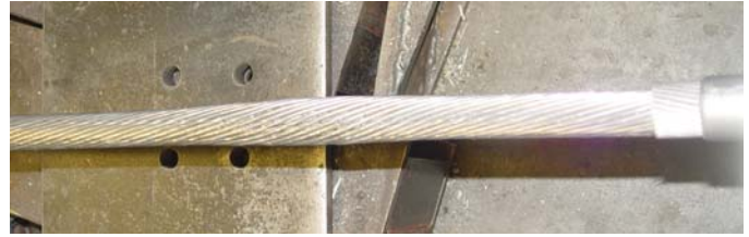
Photographs 8 and 9, bird caging of inner layer prevents conductor from returning to initial shape upon positive torque
