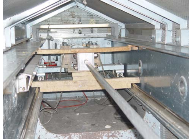
Photographs 6 and 7, initial bird cage after relaxing first negative torque cycle
