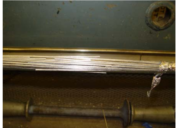
Photograph 11, core following tensile test (aluminum layers have been removed)
