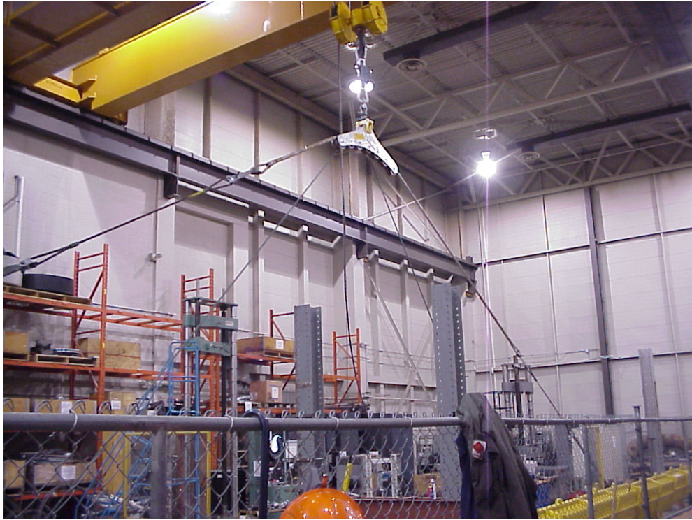
Figure 1d Typical Set-up for 7x7" Roller Array Sheave Test (60 degree break-over angle shown in photo)
