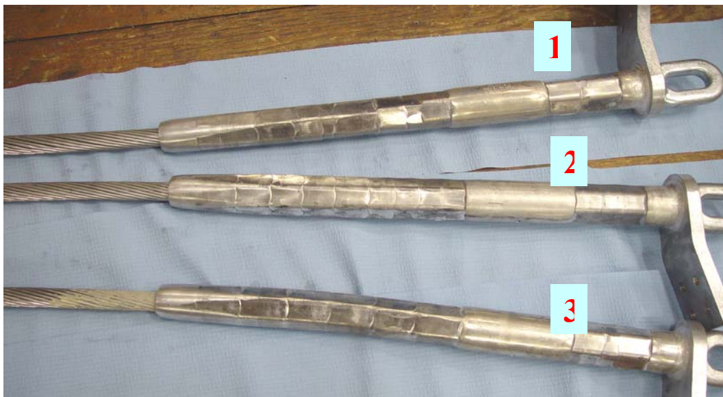
Photograph 1 , dead end samples after installation on 795 ACCR conductor (photograph courtesy of 3M Company)
