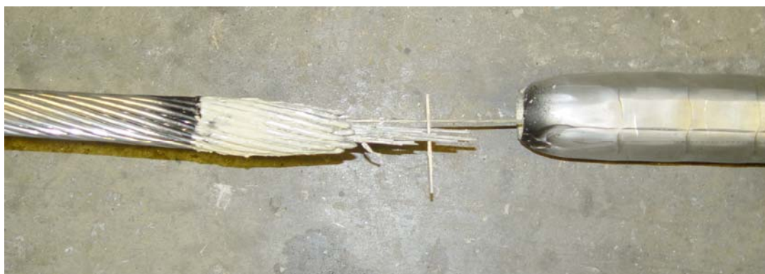
Figure 3: typical tensile overload failure
