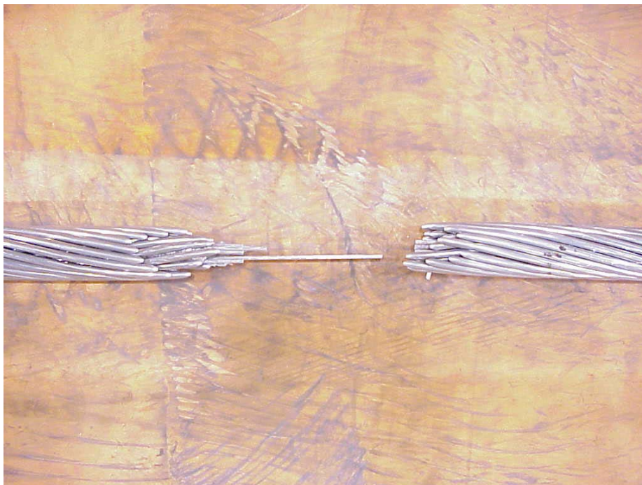
Figure 3 – “Elevated Temperature” sample after breaking
