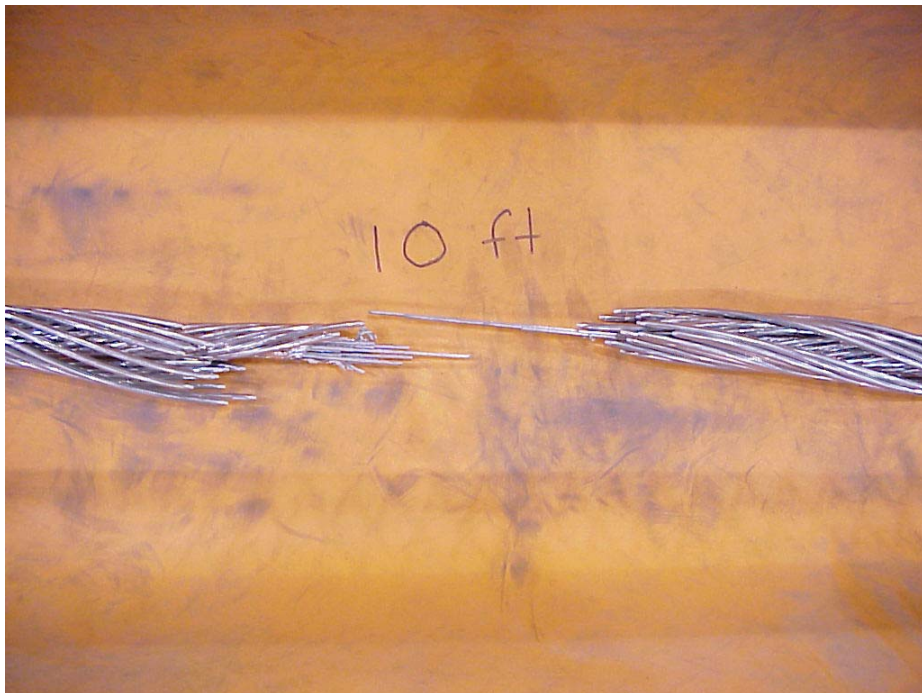
Figure 2b – “10 ft” sample after breaking
