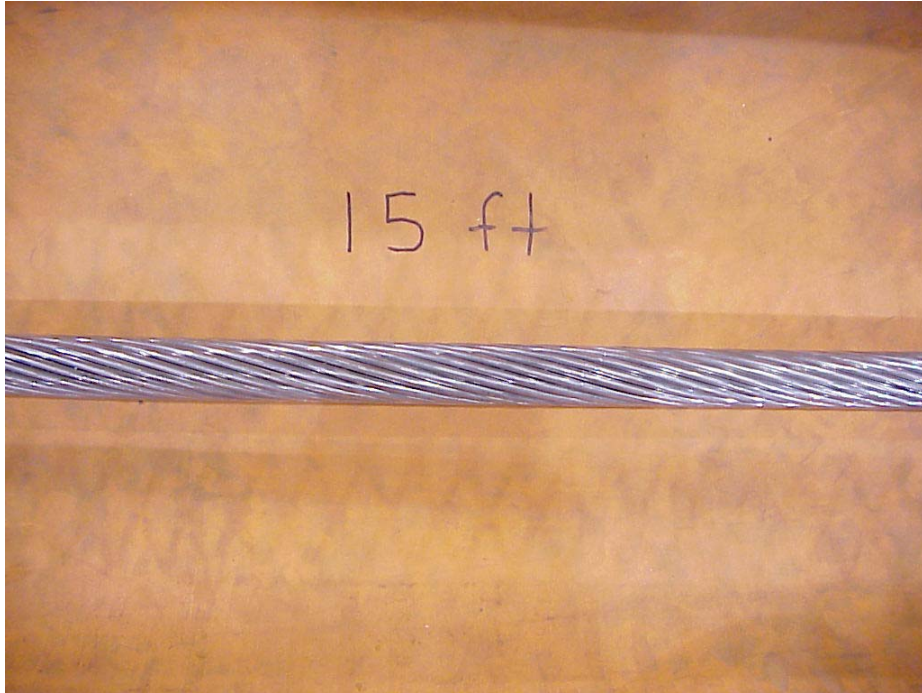
Figure 3a – “15 ft” sample before breaking
