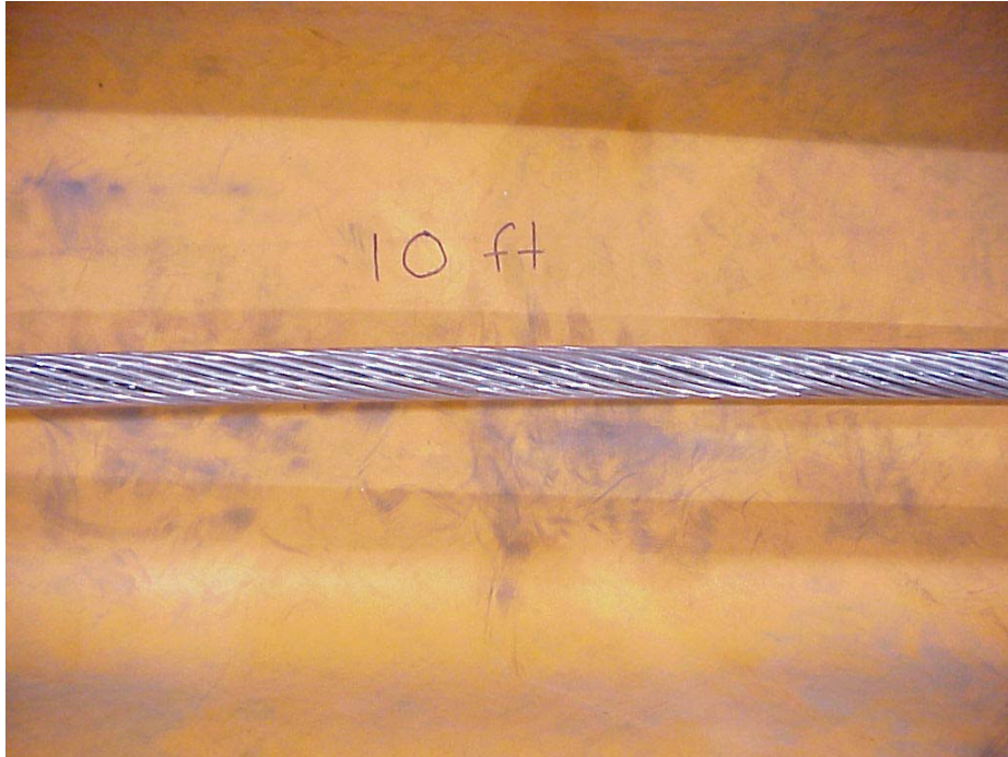
Figure 2a – “10 ft” sample before breaking
