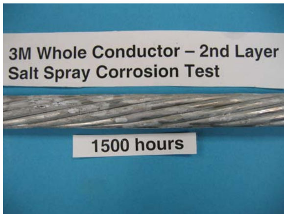
Figure 9e 3M 2nd Layer – 1500 hours AFTER Salt Corrosion Test
