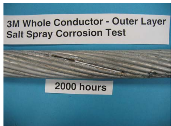
Figure 8f: 3M Outer Layer – 2000 hours AFTER Salt Corrosion Test
