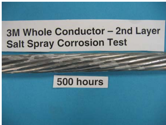
Figure 9c 3M 2nd Layer – 500 hours AFTER Salt Corrosion Test
