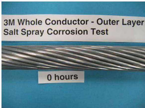
Figure 8a 3M Outer Layer – 0 hours AFTER Salt Corrosion Test
