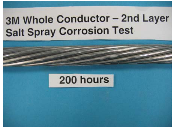
Figure 9b 3M 2nd Layer – 200 hours AFTER Salt Corrosion Test
