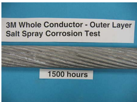
Figure 8e: 3M Outer Layer – 1500 hours AFTER Salt Corrosion Test
