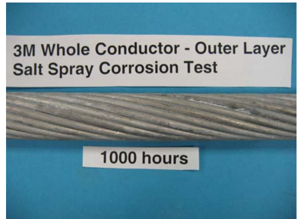
Figure 8d 3M Outer Layer – 1000 hours AFTER Salt Corrosion Test
