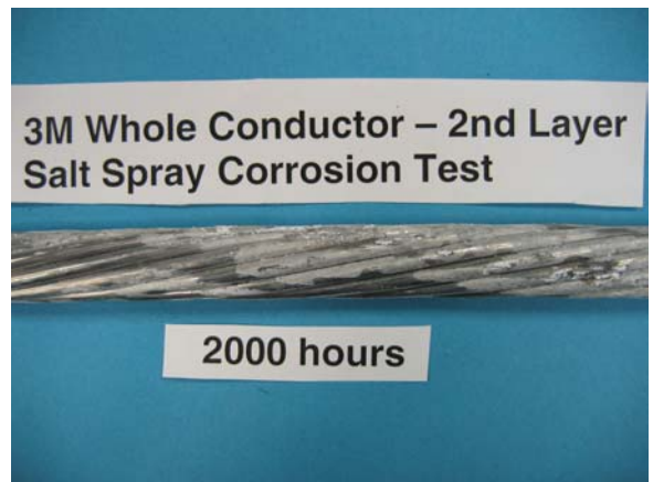
Figure 9f 3M 2nd Layer – 2000 hours AFTER Salt Corrosion Test
