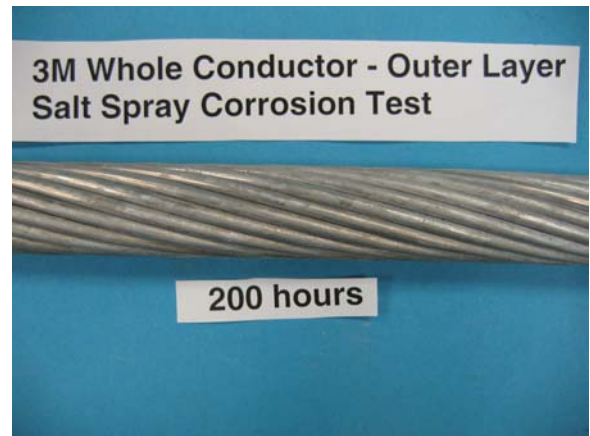
Figure 8b 3M Outer Layer – 200 hours AFTER Salt Corrosion Test
