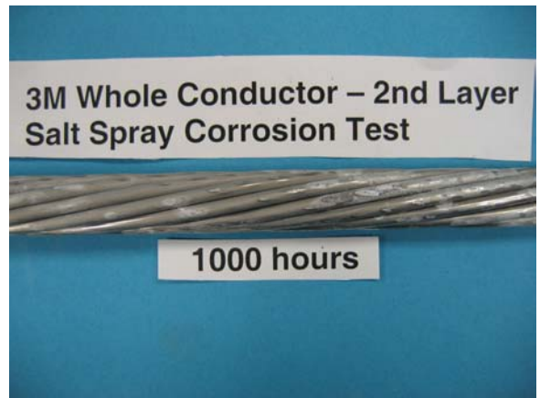
Figure 9d 3M 2nd Layer – 1000 hours AFTER Salt Corrosion Test
