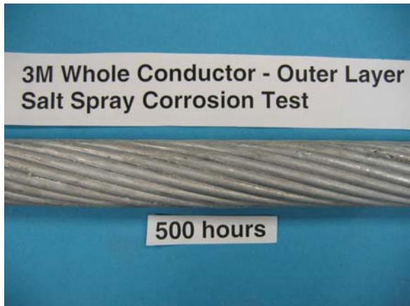
Figure 8c 3M Outer Layer – 500 hours AFTER Salt Corrosion Test
