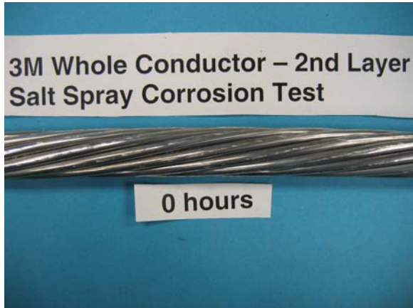
Figure 9a 3M 2nd Layer – 0 hours AFTER Salt Corrosion Test
