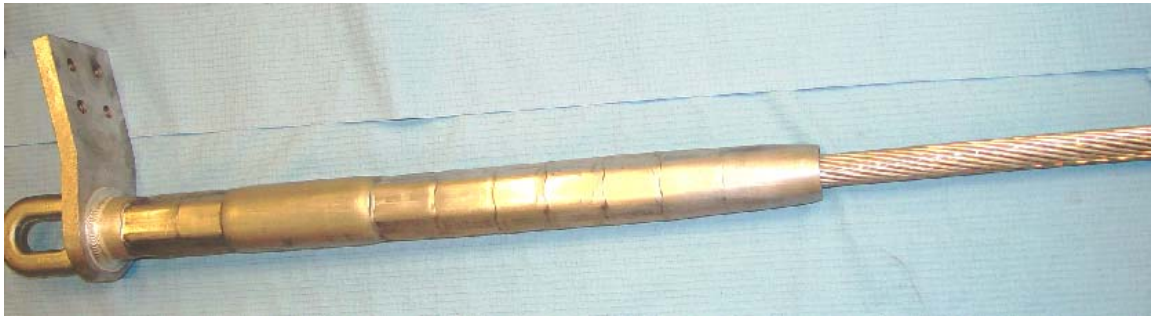
An example of a fully assembled, compression dead-end ready for testing, using the Alcoa Conductor Accessories two-piece dead-end approach.
