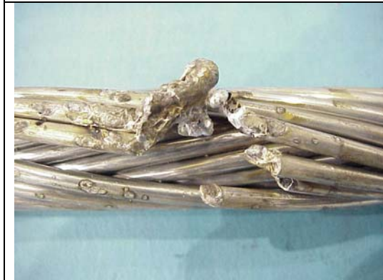
Figure A12aa – ACCR 477 kcmil, 208 C, Hit 12
