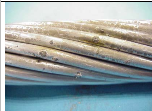
Figure B17aa – ACSR 795 kcmil, 98 C, Hit 2
