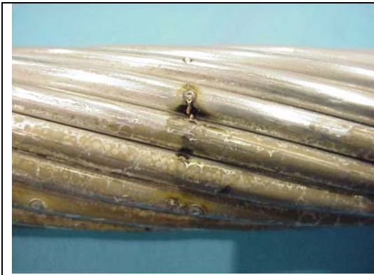
Figure B14aa – ACSR 795 kcmil, 49 C, Hit 4
