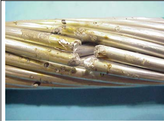
Figure B20aa – ACSR 795 kcmil, 189 C, Hit 7
