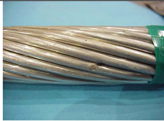
Figure B1aa – ACCR 795 kcmil, 49 C, Hit 1
