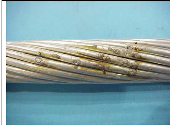
Figure A22aa – ACSR 477 kcmil, 198 C, Hit 18
