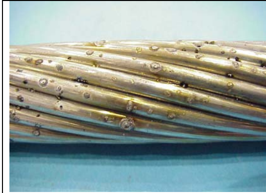
Figure B7aa – ACCR 795 kcmil, 188 C, Hit 10
