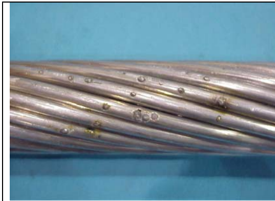
Figure B4aa – ACCR 795 kcmil, 108 C, Hit 7
