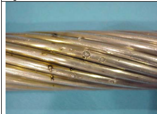
Figure B5aa – ACCR 795 kcmil, 109 C, Hit 6
