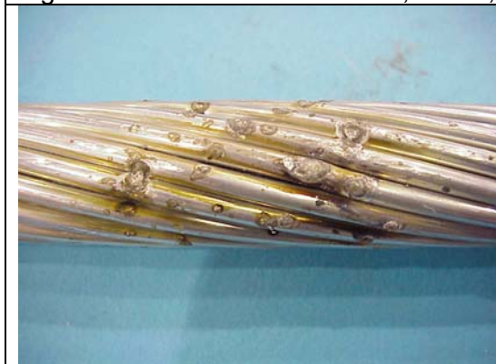
Figure A24aa – ACSR 477 kcmil, 199 C, Hit 24
