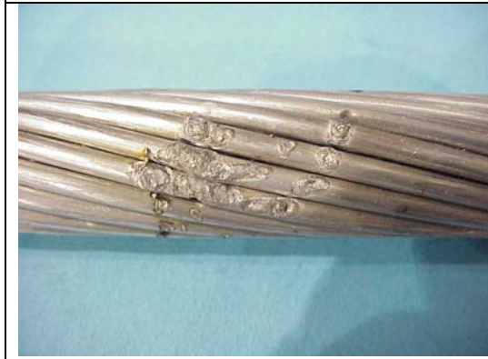
Figure A11aa – ACCR 477 kcmil, 192 C, Hit 8
