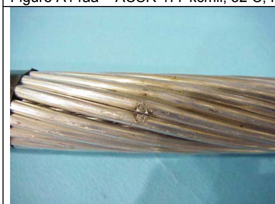
Figure A15aa – ACSR 477 kcmil, 53 C, Hit 15
