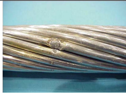
Figure B8aa – ACCR 795 kcmil, 190 C, Hit 18
