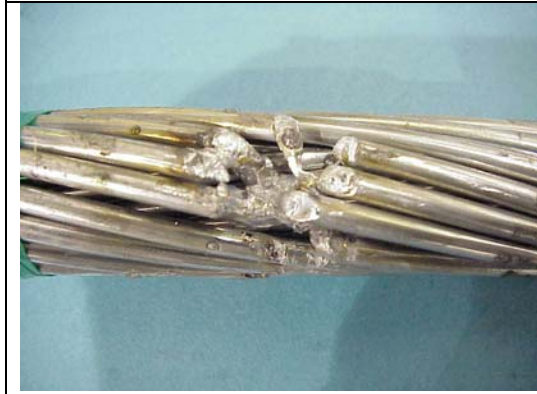
Figure A10aa – ACCR 477 kcmil, 191 C, Hit 5
