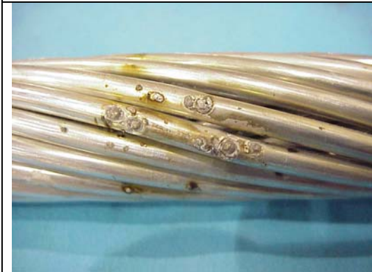
Figure B19aa – ACSR 795 kcmil, 108 C, Hit 0
