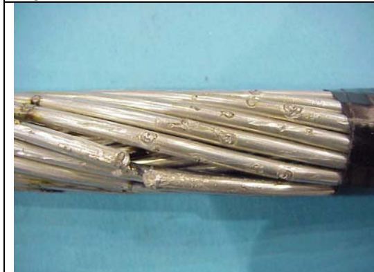
Figure A20aa – ACSR 477 kcmil, 183 C, Hit 17
