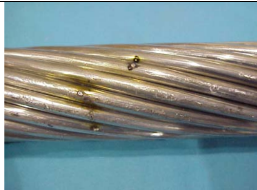
Figure B2aa – ACCR 795 kcmil, 51 C, Hit 2
