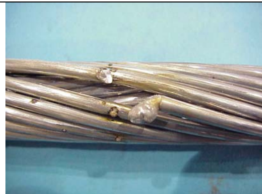
Figure A6aa – ACCR 477 kcmil, 100 C, Hit 3
