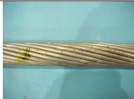
Figure A8aa – ACCR 477 kcmil, 182 C, Hit 6
