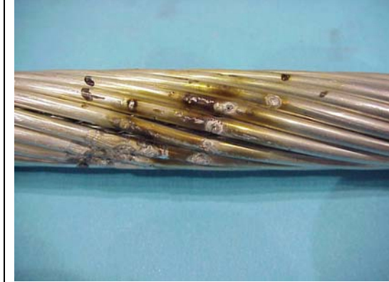
Figure A26aa – ACSR 477 kcmil, 220 C, Hit 14
