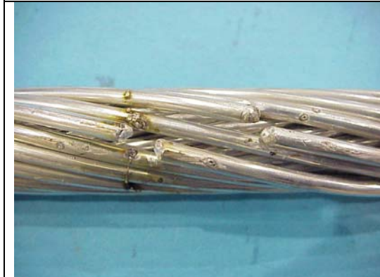
Figure A18aa – ACSR 477 kcmil, 110 C, Hit 19
