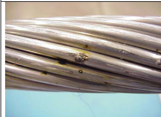
Figure B15aa – ACSR 795 kcmil, 49 C, Hit 5
