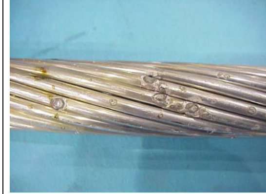
Figure A23aa – ACSR 477 kcmil, 198 C, Hit 22
