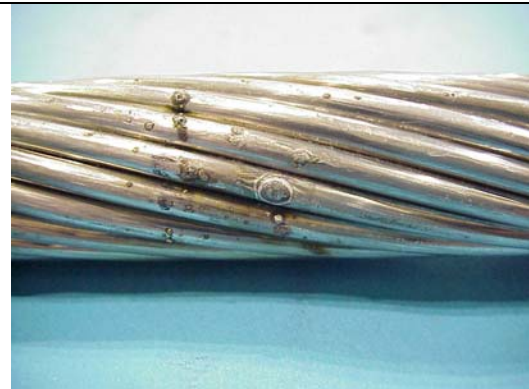
Figure B11aa – ACCR 795 kcmil, 200 C, Hit 17
