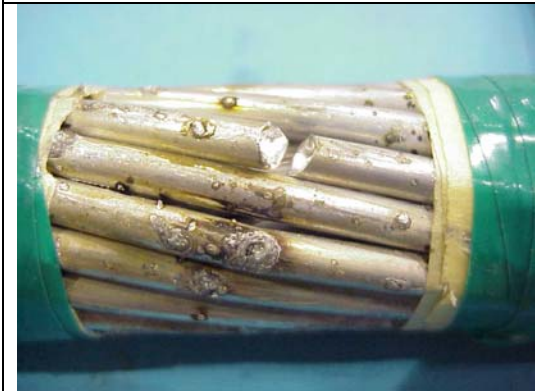
Figure B21aa – ACSR 795 kcmil, 200 C, Hit 8
