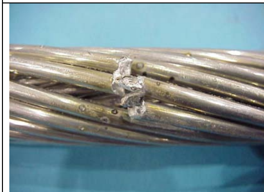
Figure B6aa – ACCR 795 kcmil, 110 C, Hit 5
