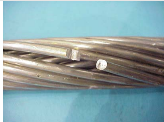
Figure A2aa – ACCR 477 kcmil, 50 C, Hit 10
