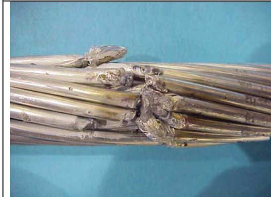
Figure A25aa – ACSR 477 kcmil, 214 C, Hit 15
