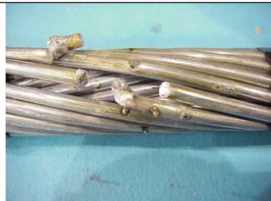
Figure A7aa – ACCR 477 kcmil, 102 C, Hit 2
