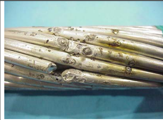
Figure B22aa – ACSR 795 kcmil, 204 C, Hit 6
