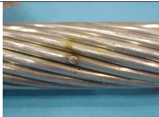
Figure B4aa – ACCR 795 kcmil, 54 C, Hit 3
