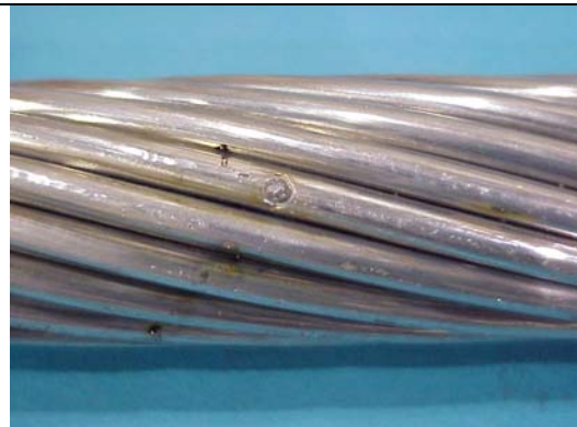
Figure B3aa – ACCR 795 kcmil, 52 C, Hit 4
