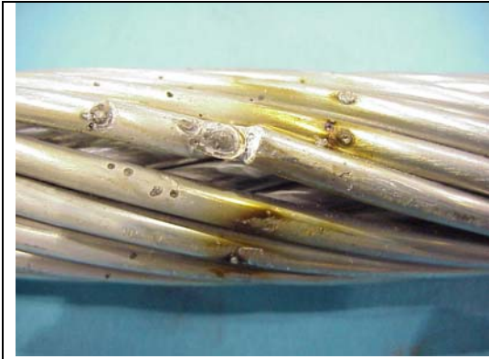
Figure B18aa – ACSR 795 kcmil, 107 C, Hit 1
