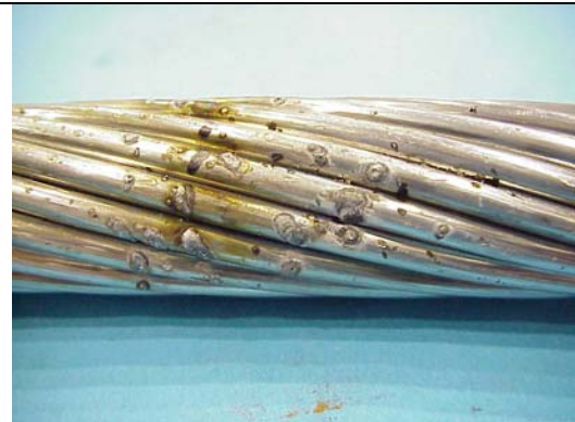
Figure B9aa – ACCR 795 kcmil, 194 C, Hit 12
