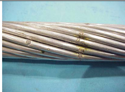
Figure A4aa – ACCR 477 kcmil, 64 C, Hit 4
