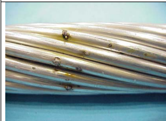
Figure B16aa – ACSR 795 kcmil, 50 C, Hit 3
