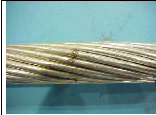
Figure A14aa – ACSR 477 kcmil, 52 C, Hit 13
