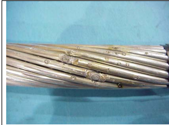
Figure A21aa – ACSR 477 kcmil, 189 C, Hit 23
