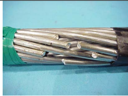
Figure A5aa – ACCR 477 kcmil, 90 C, Hit 1
