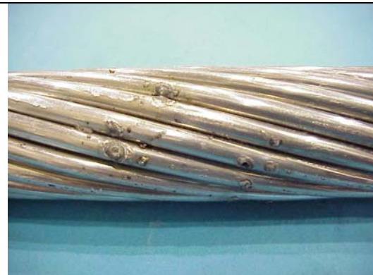
Figure B10aa – ACCR 795 kcmil, 196 C, Hit 9
