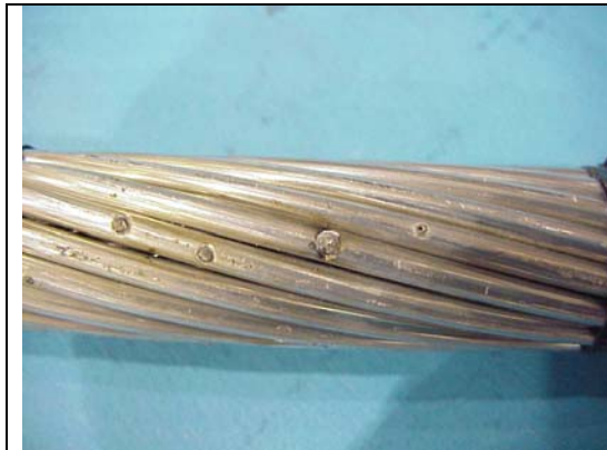
Figure A13aa – ACSR 477 kcmil, 48 C, Hit 14
