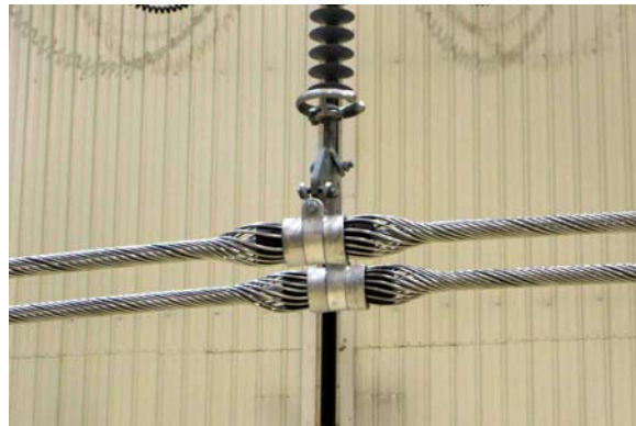
Figure 4 – Corona Test Arrangement
