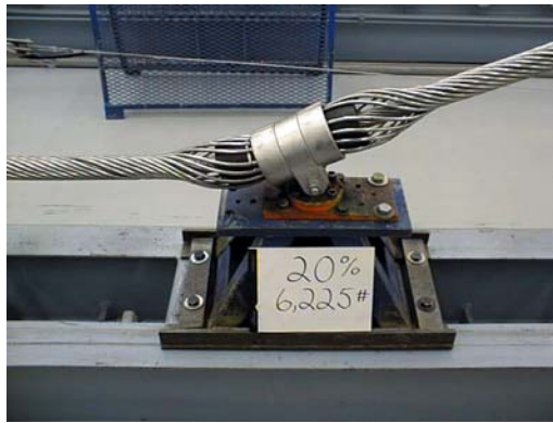
Figure 2 – Unbalanced Load Test Arrangement
