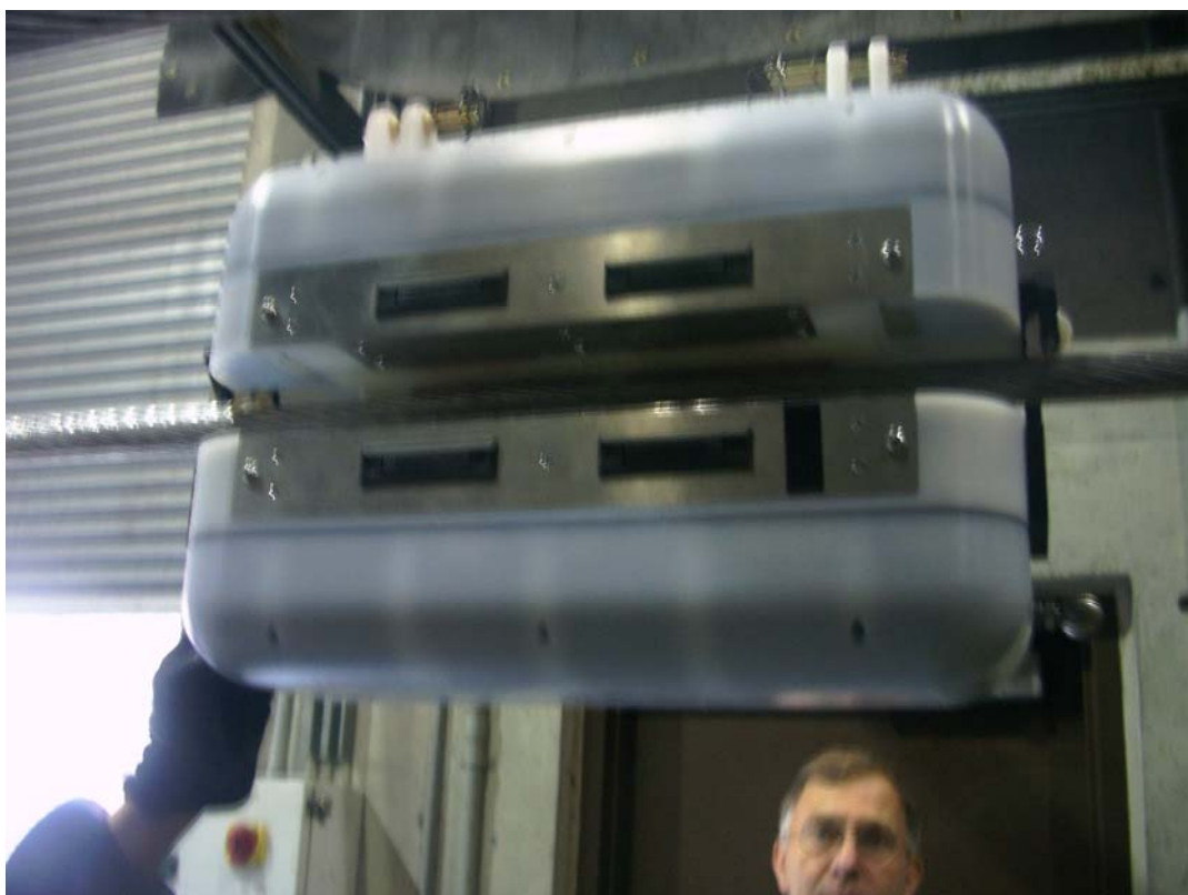
Figure 3a: EMAT Device (Open Position for Installing on Conductor)
