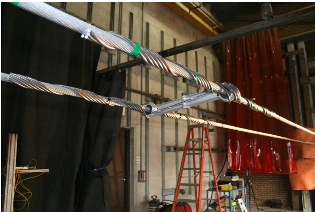
Figure 2: PLP Rigid Spacer and Rods Installed at Mid-Span on 2 x 795 ACCR Conductors
