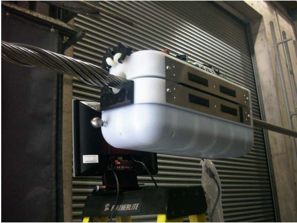
Figure 3b: EMAT Device (Closed Position for Taking Measurement)
