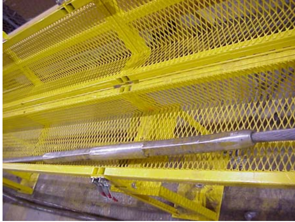
Figure 3a: 1272 kcmil Full Tension Splice after Tension Test at Room Temperature (Sample #3)
