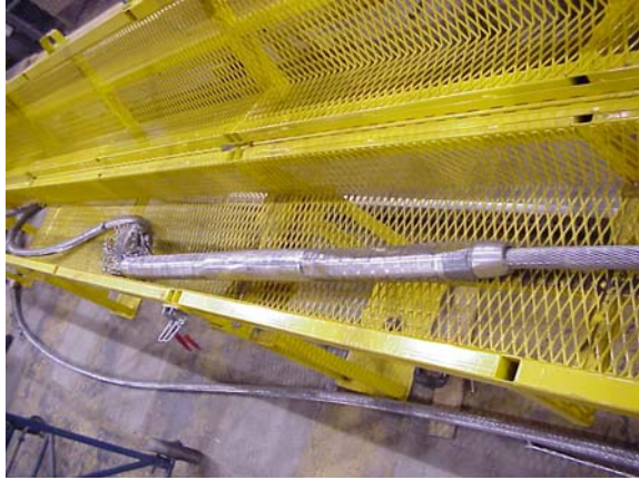
Figure 2a: 1272 kcmil Full Tension Splice after Tension Test at Room Temperature (Sample #2)
