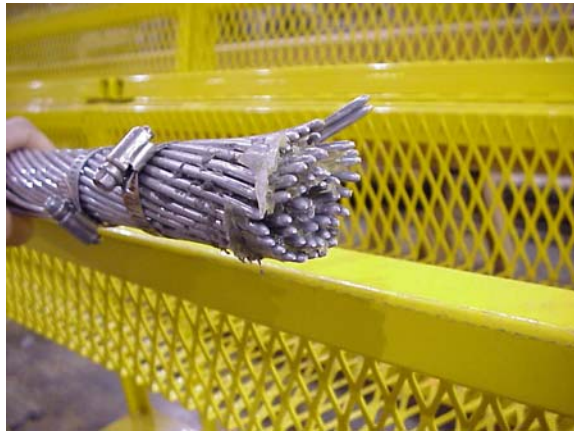
Figure 2a: Failed 1272 kcmil Conductor after Tension Test at Room Temperature (Sample #2)
