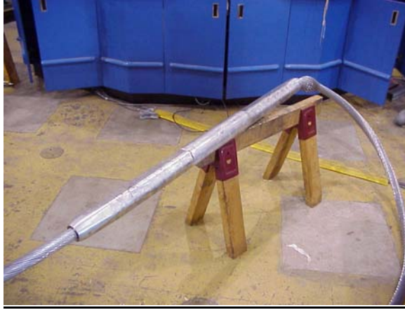
Figure 1a: 1272 kcmil Full Tension Splice after Tension Test at Room Temperature (Sample #1)
