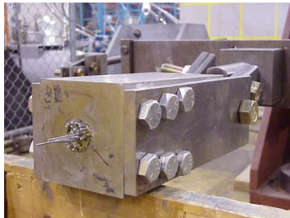
Figure 1c: 1272 kcmil Conductor at North Epoxy-Resin Clamp Location after Tension to Failure Test at Room Temperature (Sample #1)
