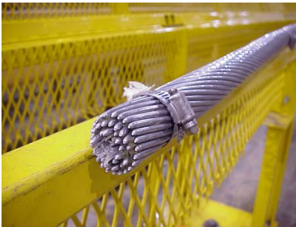
Figure 3a: Failed 1272 kcmil Conductor after Tension Test at Room Temperature (Sample #3)
