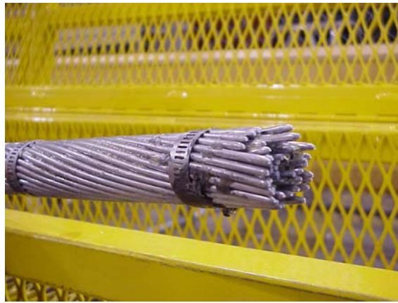
Figure 1b: Failed 1272 kcmil Conductor after Tension Test at Room Temperature (Sample #1)
