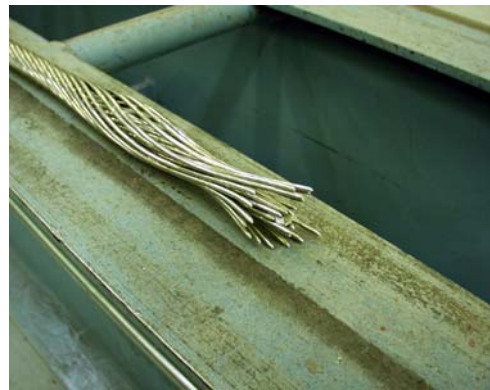
Figure 2 – Typical Mid-Span Failure
