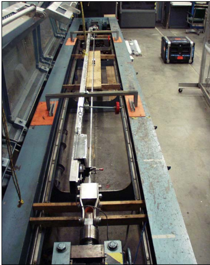
Photograph 1, Long View of Stress-Strain Test (conductor shown is 477 ACCR, not sample from this project)
