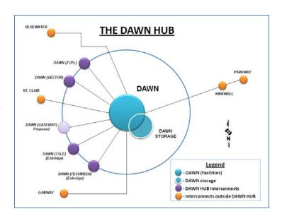
place at the center – "Dawn". This is where storage injections and withdrawals occur and where the Union Gas Dawn to Parkway system originates. The other locations within the Dawn Hub facilitate the transportation between interconnecting pipelines and the Dawn trading and storage center.
