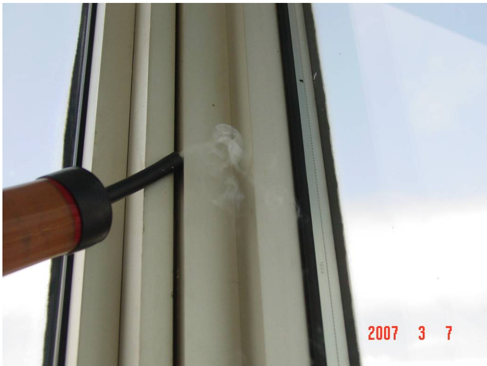
Photograph 26: The gaps or openings and the lack of sealant between the window framing components allows cold air to enter the building at these locations.
