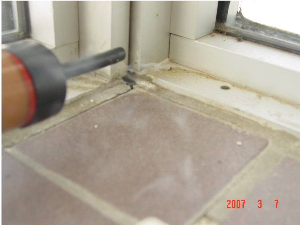
Photograph 25: Using a smoke pencil, it was observed at various locations at the window framing gaps and openings, that air leakage was evident.
