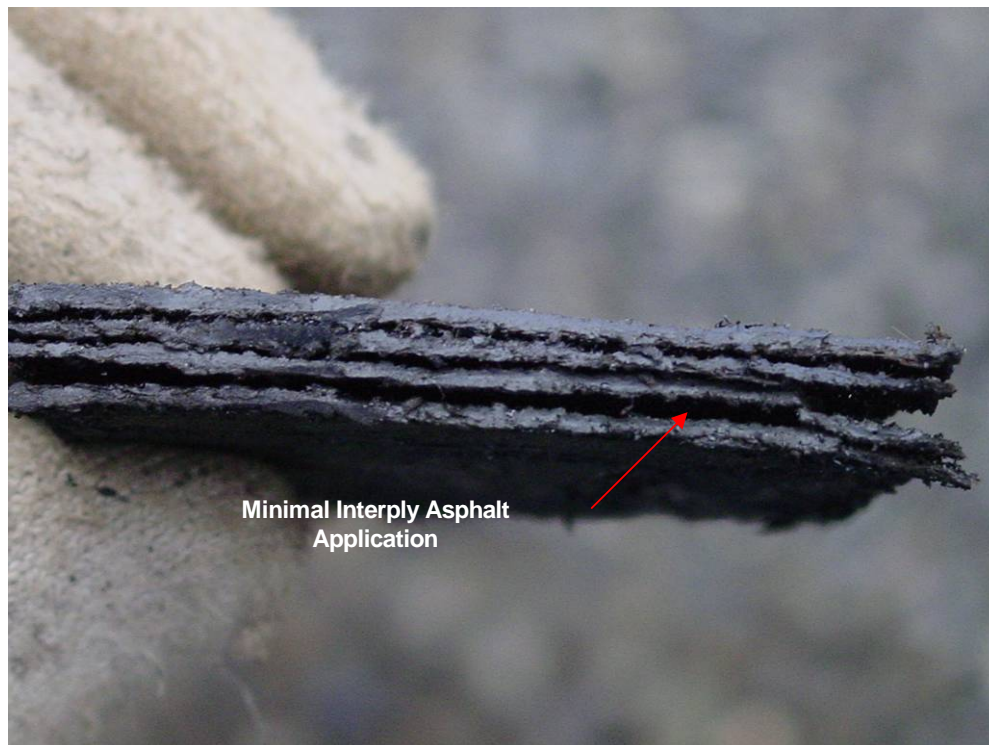
Photograph 52: Roof Area 4.1 – The existing membrane exhibits very poor interply adhesion.
