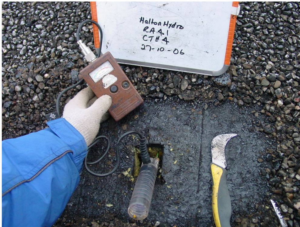
Photograph 51: Roof Area 4.1 - Probes taken at the core cut locations revealed no moisture present in the insulation layer or within the membrane interply.
