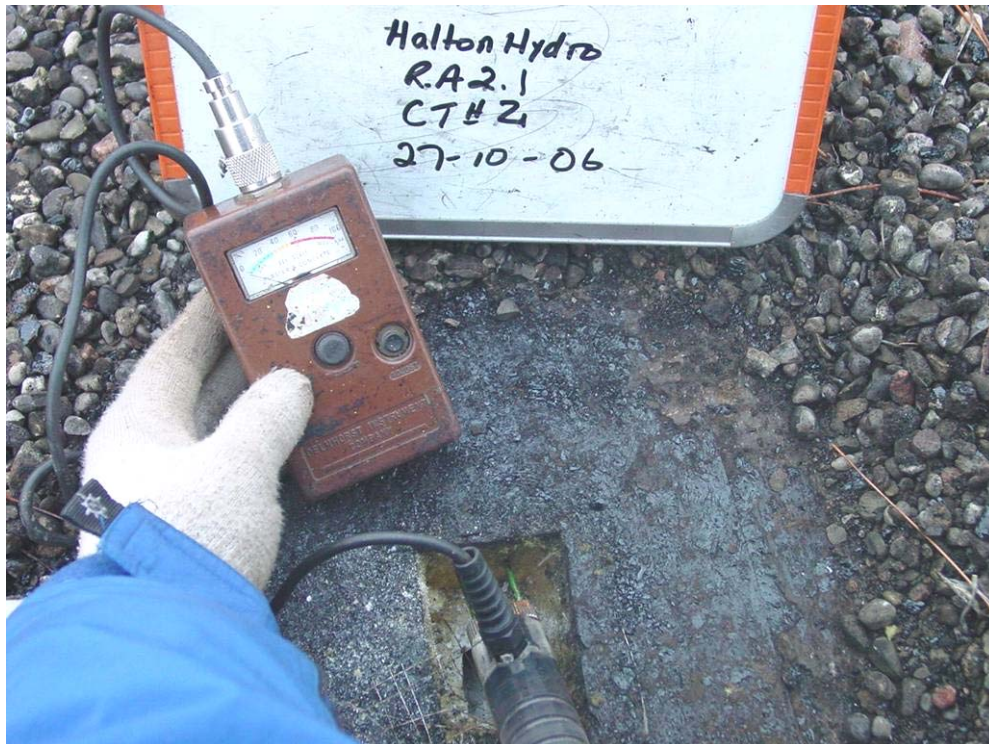
Photograph 23: Roof Area 2.1 – Probes taken at the core cut locations revealed no moisture present in the insulation layer or within the membrane interply.
