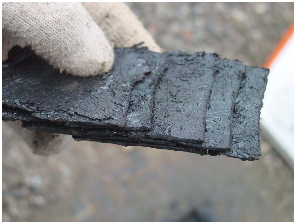
Photograph 24: Roof Area 2.1 – The membrane at the core cut on this area exhibits very poor interply adhesion. The individual membrane plies were very easily delaminated.
