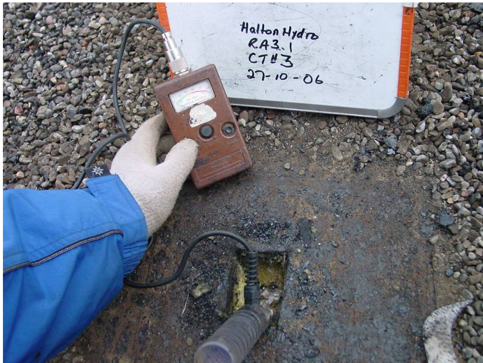
Photograph 41: Roof Area 3.1 – Core cuts revealed that the membrane is exhibiting top ply deterioration in addition to weak interply adhesion due to inadequate asphalt application quantities. Probes taken at the core cut locations revealed no moisture present in the insulation layer or within the membrane interply
