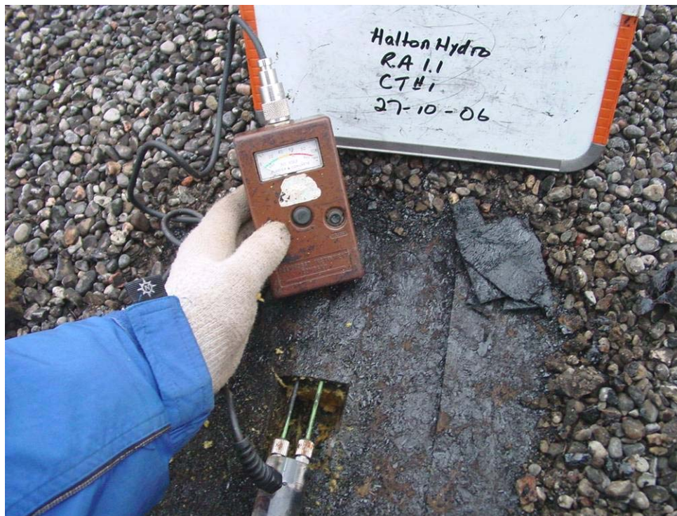
Photograph 6: Roof Area 1.1 – Core cuts revealed that the membrane is exhibiting top ply deterioration, increased brittleness and poor interply adhesion. These observations would suggest that the existing membrane is in poor condition with limited service life remaining. Probes taken at the core cut locations revealed no moisture present in the insulation layer or within the membrane interply.
