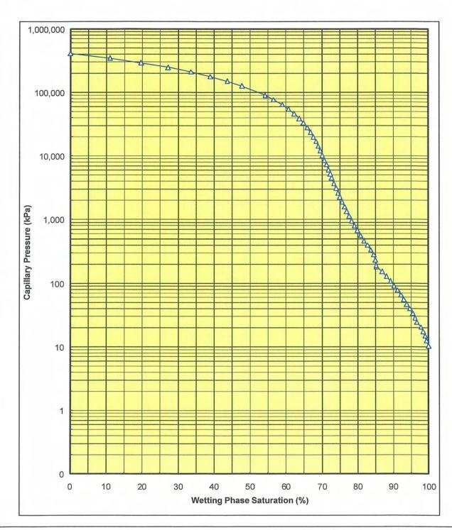
Figure 1B: Derived Air/Water Capillary Pressure vs. Wetting Phase Saturation – SP-1
