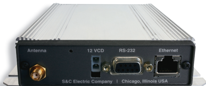
Antenna, power, and serial and Ethernet data input connections on SpeedNet Radio.
