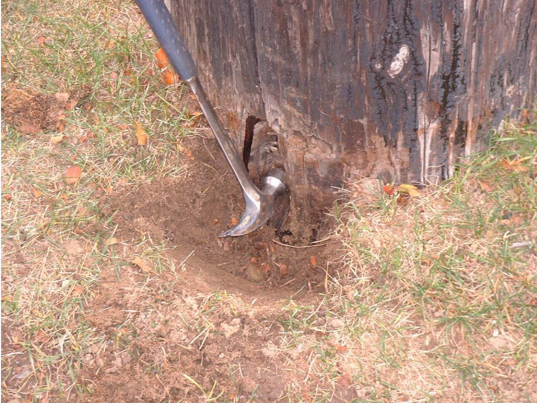
Picture 2: Hammer test of rot below ground level.
