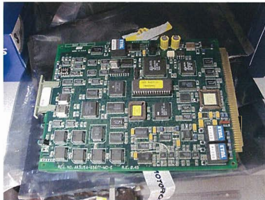
Figure 1 – Existing Globalview Serial Modem
