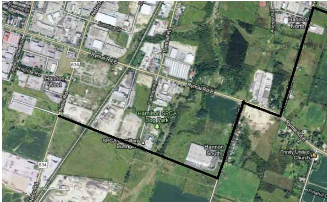
Figure 5: Express circuit indicated in black. The express circuits continue eastward from the NEBO TS along the HONI transmission corridor until they meet Glover Road. As the feeders turn north along Glover Road, they enter Horizon Utilities' service area. The point of demarcation between HONI and Horizon Utilities in respect of these feeders is located approximately at the top right corner of the above figure.
