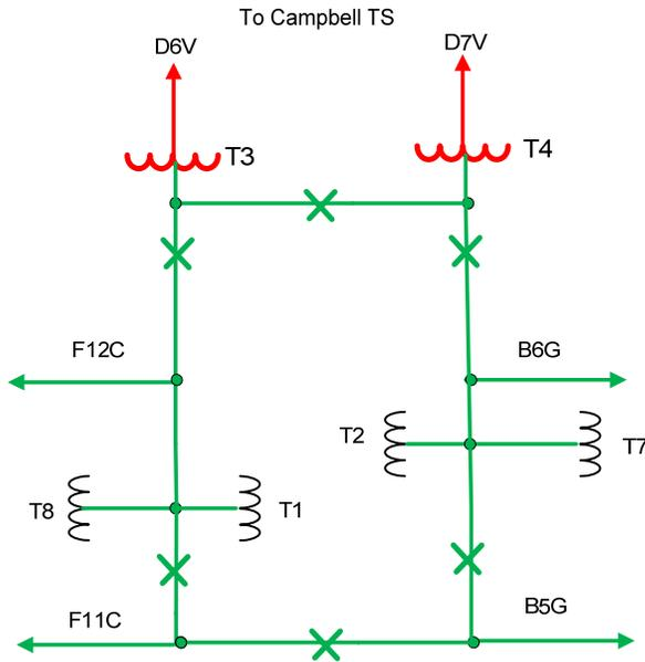
**Figure 5: STAGE 2 - Schematic Single Line Diagram CEDAR TS ring bus configuration with six 115 kV breakers (future configuration - ultimate design)**
