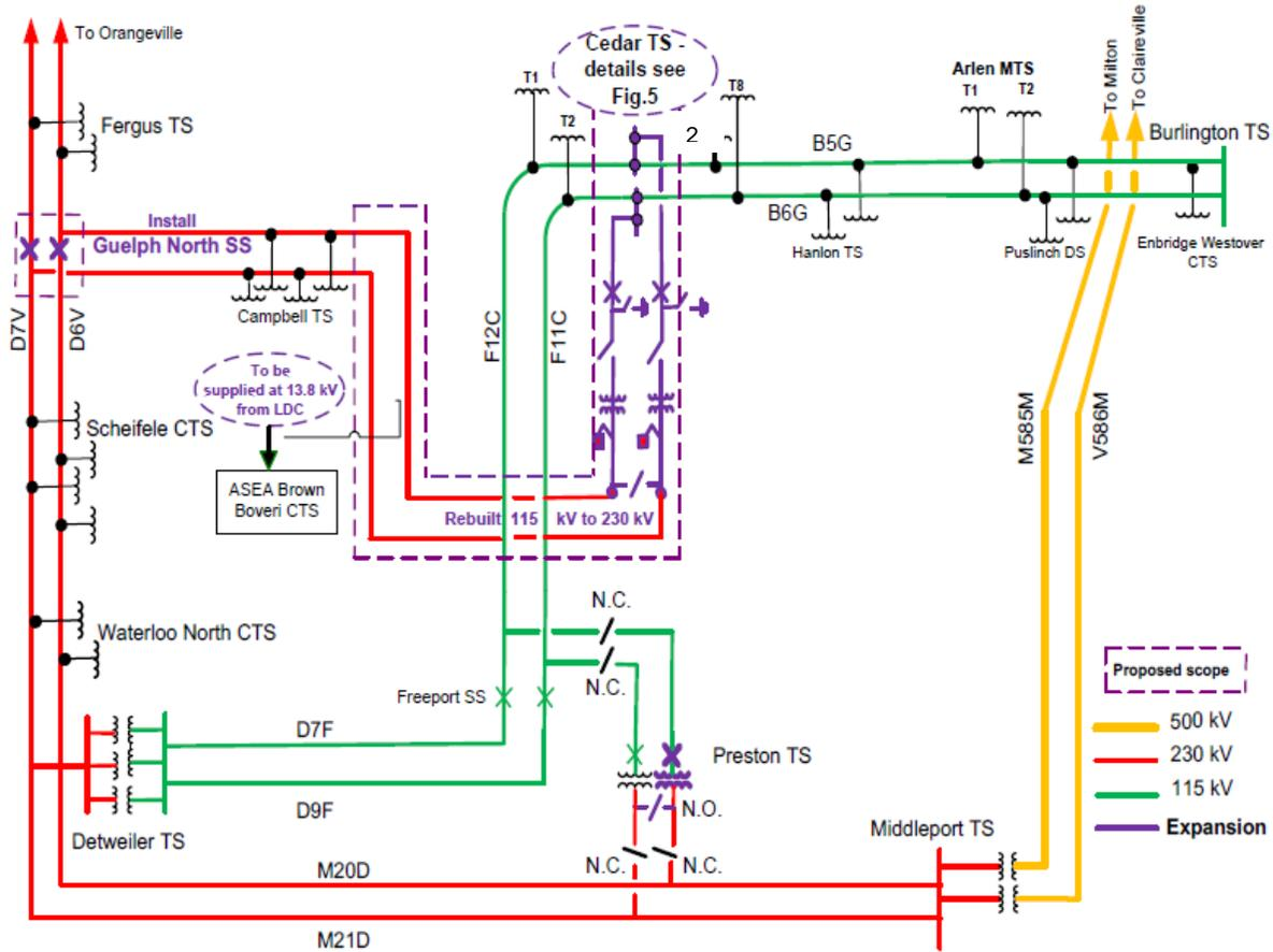
**Figure 1** : Install two 230/115 kV autotransformers at Cedar TS, 2 in-line breakers at Guelph North Junction and 2 in-line breakers at Cedar TS
