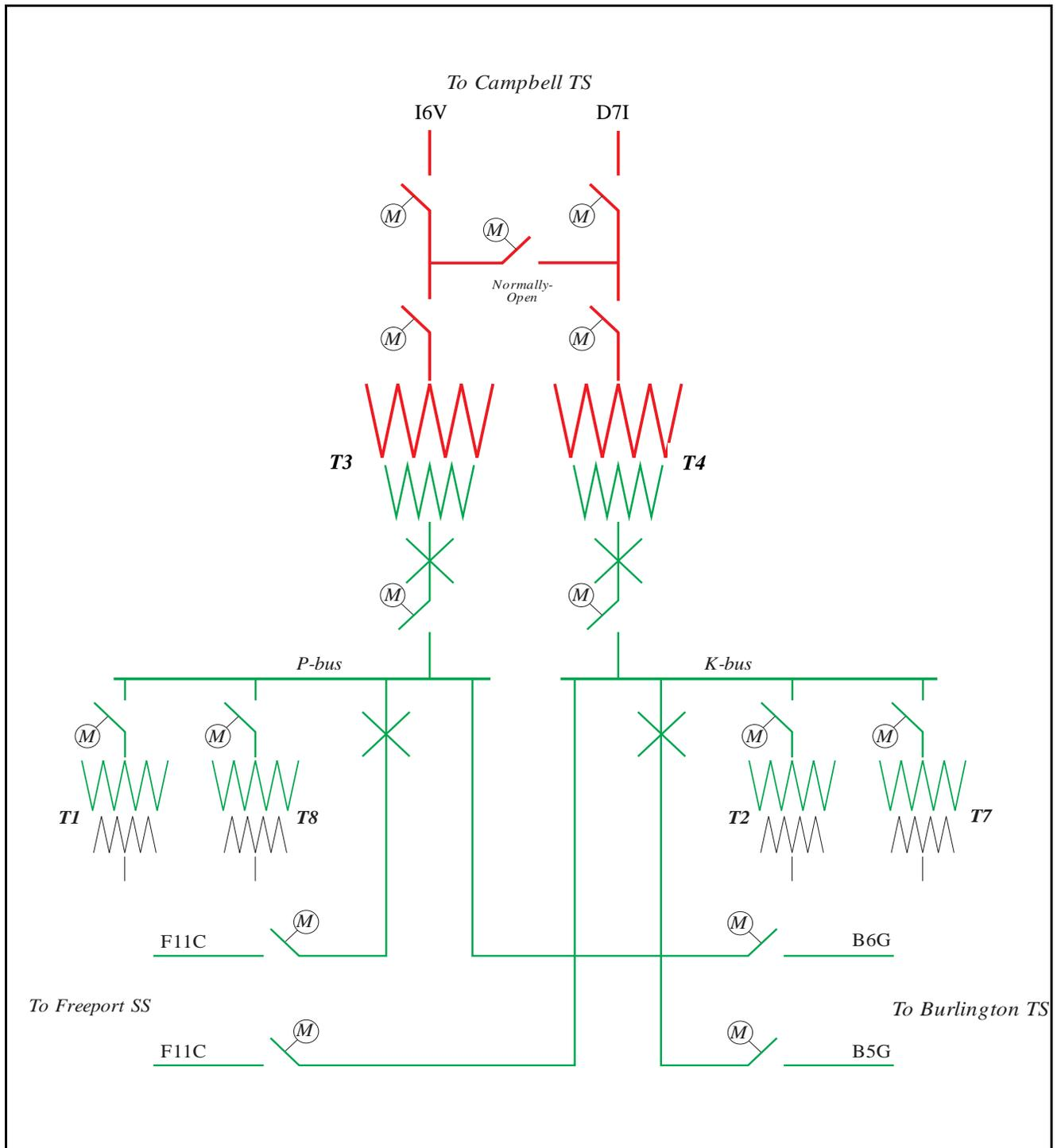
**Figure 4: Hydro One Proposed Cedar TS Configuration**
