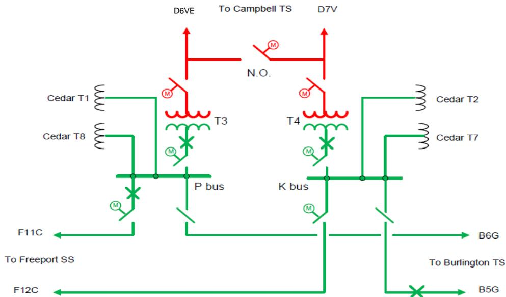
**Figure 2** – Configuration of 2 in-line breakers (staggered) at Cedar TS
